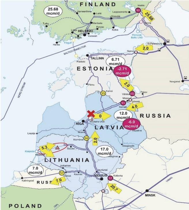
Fig. 3.2. Natural gas flows in natural transmission system of the Baltic States and Finland in case of supply disruption from Inčukalns USG (base scenario)<sup>7</sup>, where
