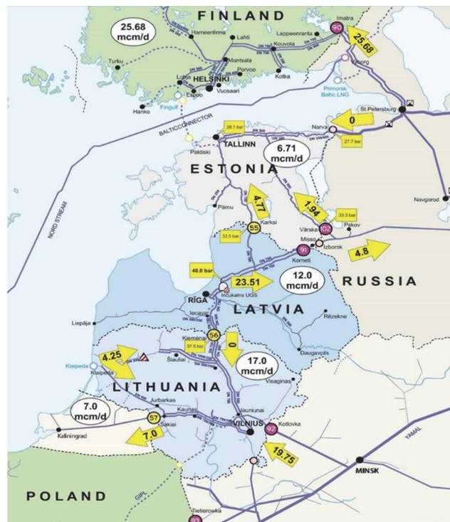
Fig. 3.1. Existing natural gas flows in natural gas transmission systems of the Baltic States and Finland in normal conditions<sup>6</sup>, where
