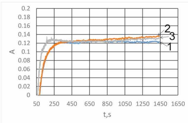
**Fig.12.** PA contrast versus time in the case of  $p-p$  recording. Transmission mode.
