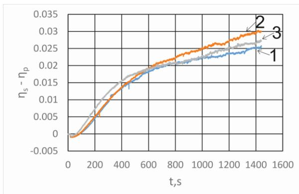
**Fig.14.** DE difference versus time in the case of  $p-p$  recording. Transmission mode.
