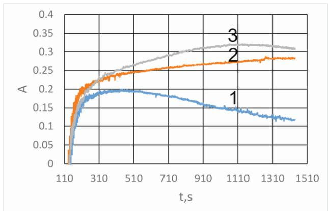
**Fig.13.** PA contrast versus time in the case of  $p-p$  recording. Reflection mode.
