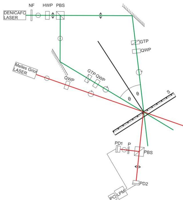
**Fig.2.** Experimental setup for transmission mode PA measurements. Notations are explained in the text.
