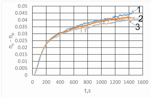
**Fig.10.** DE difference versus time in the case of  $L-R$  recording. Transmission mode.
