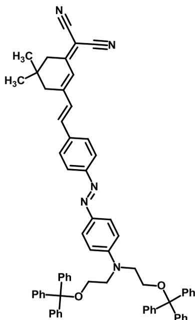
**Fig.1.** Chemical structural formula of IWK-2D film. It has *trans*-absorption maximum at 500 nm and glass transition temperature  $T_g = 105^{\circ}\text{C}$ .
