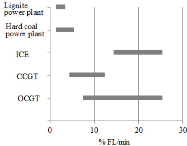
Fig. 2.18. The ramping capability of different technologies (developed by the author according to [19]); (Installed capacity of power plants: lignite: 500–1000 MW; CCGT: 300–500 MW; OCGT: 20–200 MW; ICE: 20–200 MW).
