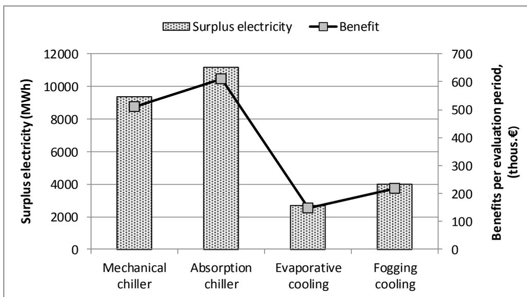
Fig. 6.6. Additional electricity and benefits of different air cooling technologies [98].
