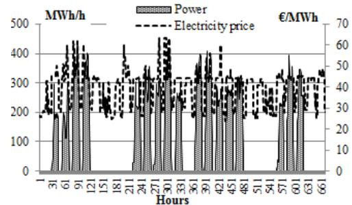
Fig. 2.2. Electricity generation profile of Riga TPP–2 plant from 1 February 2015 to 28 February 2015 [4].
