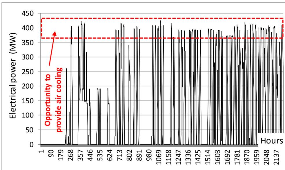
Fig. 6.4. Example of CCGT–2/2 unit operation in summer (June–August) in 2015 [98].
