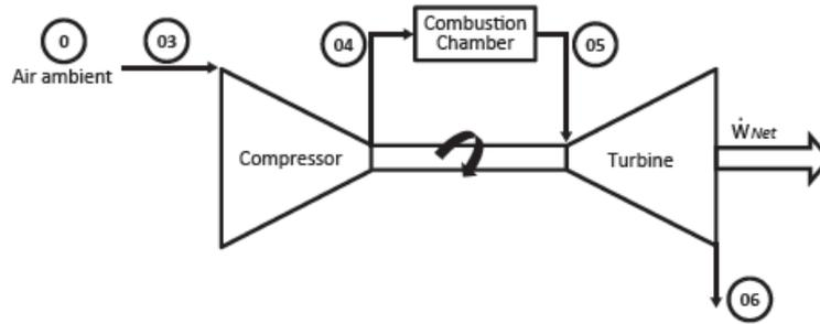
Fig. 6.2. Gas turbine unit (0, 03, 04, 05, 06 refer to a lower index in the equations below) [85].
