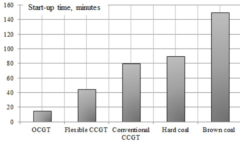
Fig. 2.16. The duration of hot start-up time of different technologies (developed by the author according to [19]).
