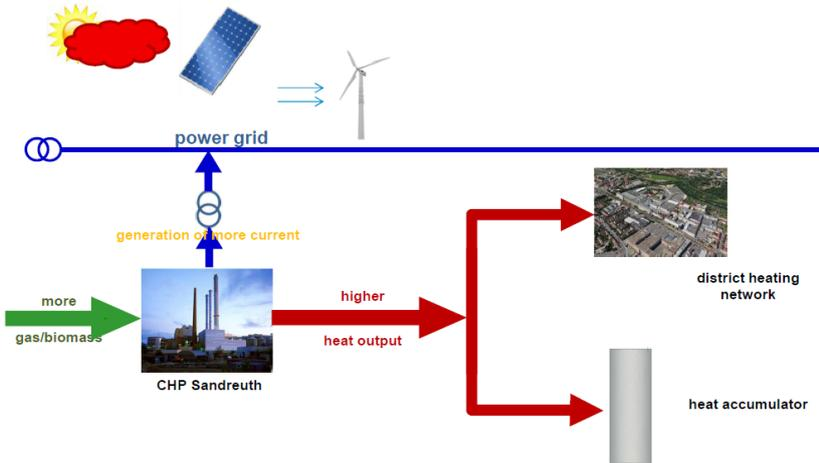
Fig. 2.3. The operation of *Sandreuth* TPP, when the intermittent generation is not available [18].
