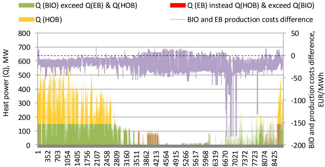
Fig. 7.7. Operation of the electric boiler in line with *Target No. 2* [59].
