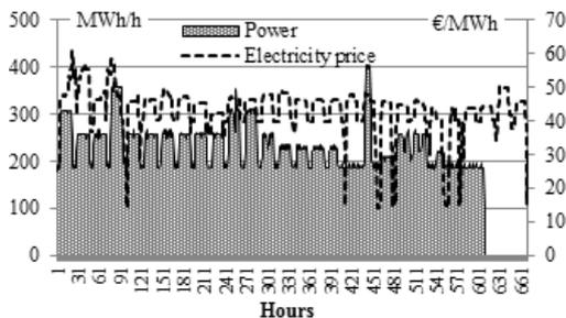
Fig. 2.1. Electricity generation profile of Riga TPP–2 plant from 1 February 2013 to 28 February 2013 [4].
