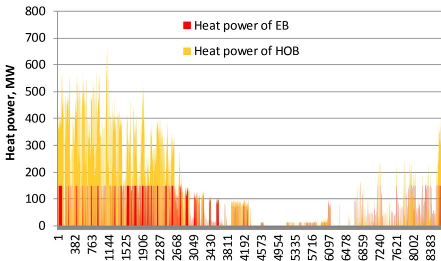
Fig. 7.6. Operation of the electric boiler in line with *Target No.1* [59].
