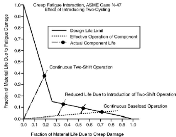
Fig. 2.8. Creep and fatigue interaction [13].
