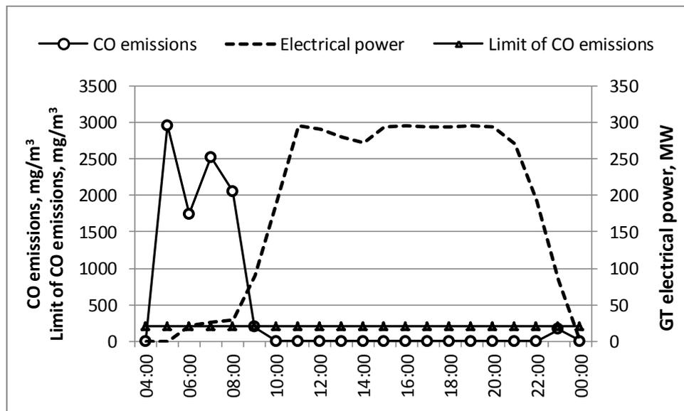
Fig. 2.27. CO emissions during the start-up procedure [24].
