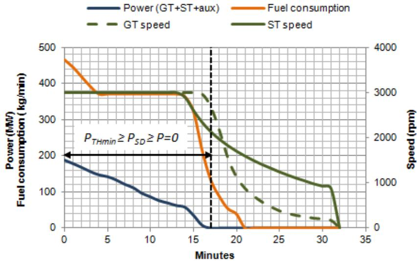
Fig. 3.2. Shutdown of production unit CCGT-2/2 [63].
