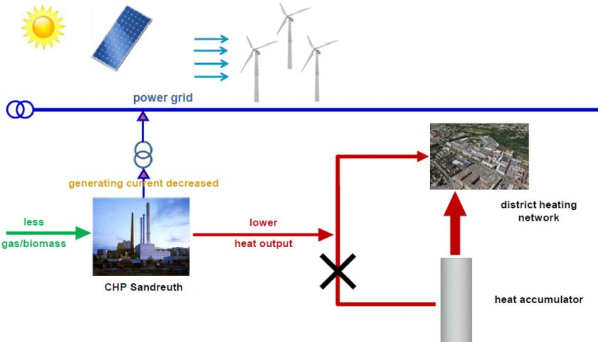
Fig. 2.4. The operation of *Sandreuth* TPP, when the intermittent generation is available [18].
