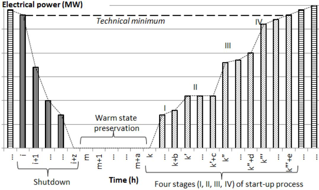
Fig. 3.1. The illustration of transient modes (one cycle) [63].
