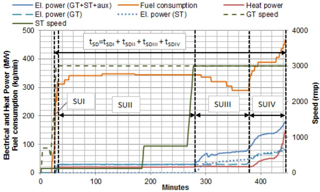
Fig. 3.3. Start-up of CCGT-2/2 unit [63].
