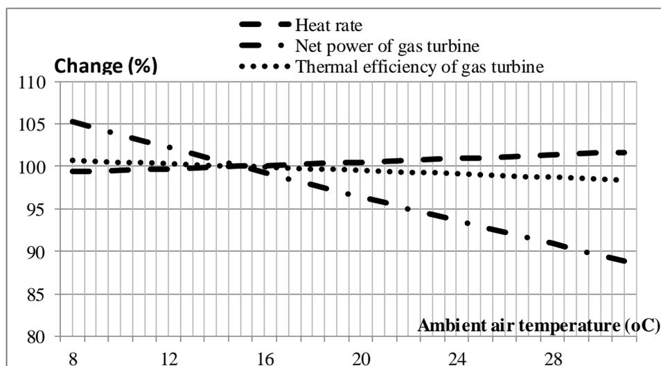
Fig. 6.3. The influence of ambient air temperature on 9F.05 GT unit performance [98].
