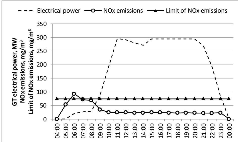
Fig. 2.26. NO<sub>x</sub> emissions during the start-up procedure [24].
