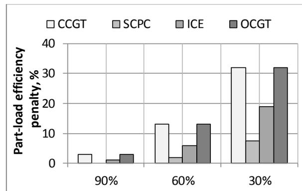
Fig. 2.15. Part-load efficiency penalty for different technologies (developed by the author according to [19]) (OCGT approx. 100 MW; CCGT – 120 MW; ICE – 20 MW; SCPC – 1 GW).
