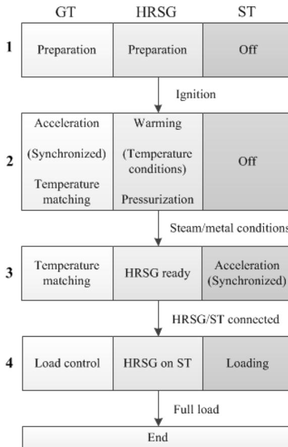
Fig. 2.6. Start-up procedure of CCGT power plant (developed by the author according to [21]).
