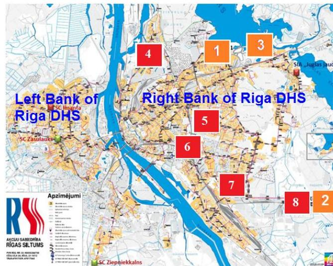
Existing heat energy sources in the right bank DHS: 1) Riga TPP–1;  $Q=493$ ;  $P=144$  MW; fuel – natural gas; 2) Riga TPP–2;  $Q=1124$ ;  $P=832$  MW; fuel – natural gas; 3) TPP *Juglas jauda*;  $Q=16$ ;  $P=14.9$  MW; fuel – natural gas.
