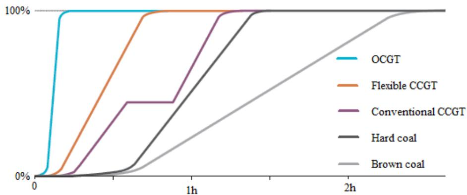
Fig. 2.17. The start-up trajectories of different technologies [19].
