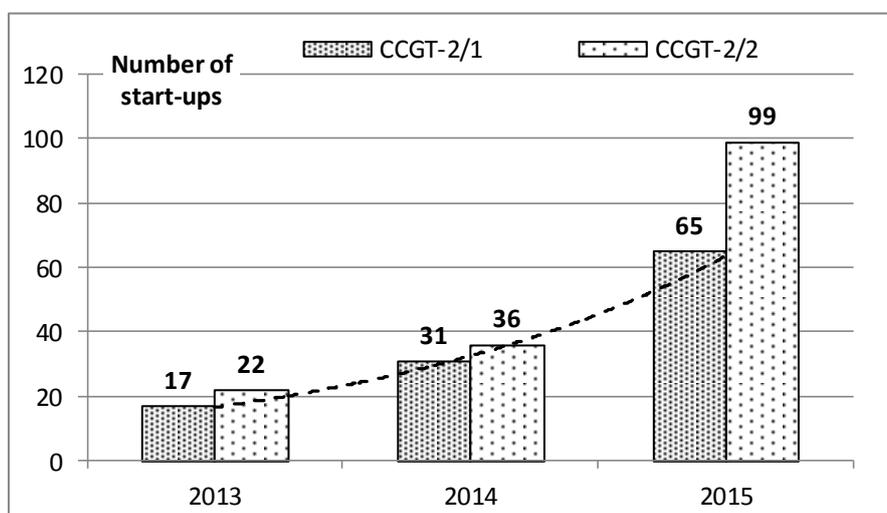
Fig. 2.25. The number of start-ups of CCGT–2/1 unit and CCGT–2/2 unit in 2013, 2014, 2015 [24].
