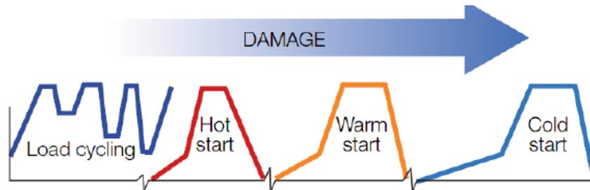
Fig. 2.7. The types of cycling operation [13].
