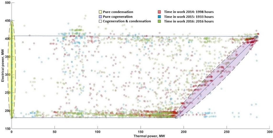
Fig. 2.23. Statistics of CCGT–2/1 unit operation [58].
