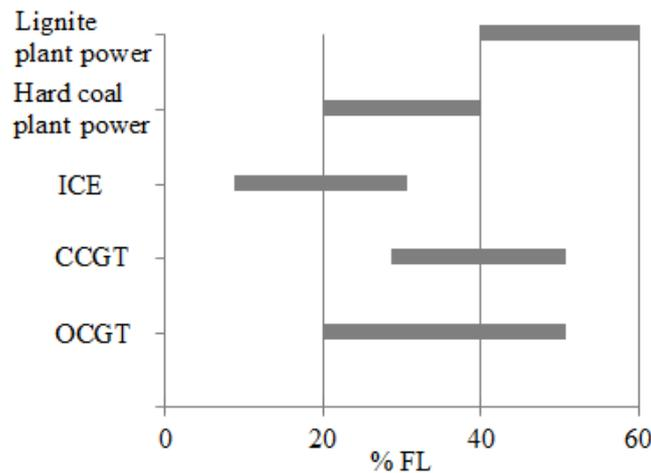
Fig. 2.19. The minimum turndown of different technologies (developed by the author according to [19]); (Installed capacity of power plants: lignite: 500–1000 MW; CCGT: 300–500 MW; OCGT: 20–200 MW; ICE: 20–200 MW).
