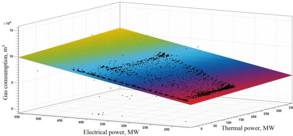
Fig. 4.4. Consumption of natural gas as a function of electrical and heat power [58].
