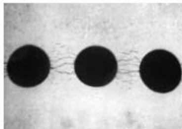
Fig. 2.9. Cracking seen from inside of the economizer header [13].
