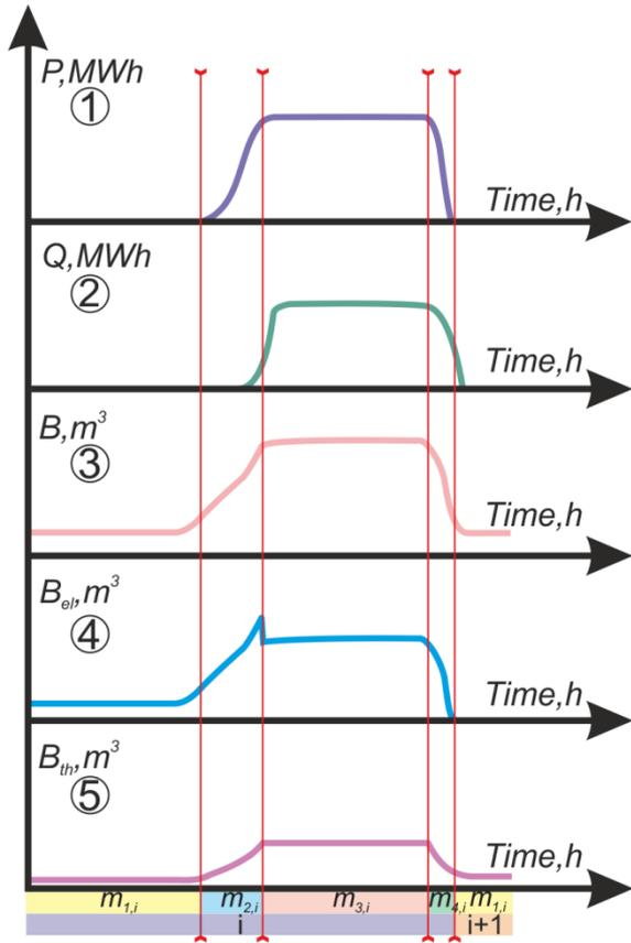
Fig. 4.3 The schematic change in electricity, heat and fuel during the cycling operation range “*i*” [58].
