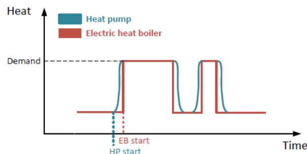
Fig. 7.2. Ramping principles of heat pump and electric boiler [111].
