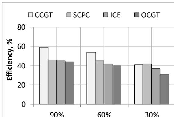
Fig. 2.14. Efficiency versus load for different technologies (developed by the author according to [19]) (OCGT approx. 100 MW; CCGT – 120 MW; ICE – 20 MW; SCPC – 1 GW).
