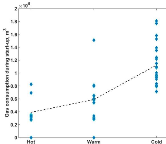
Fig. 4.8. The consumption of natural gas versus the start-up type [58].
