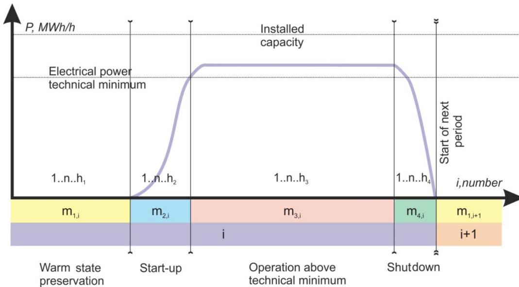
Fig. 4.2 The model of cycling operation range ( $i$ ) [58].
