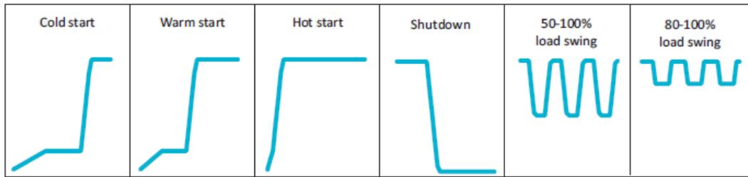
Fig. 2.5. Type of cycling operation [19].
