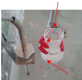
Fig. 2.1. Eutectic mixture in constant temperature water bath with thermocouples.
