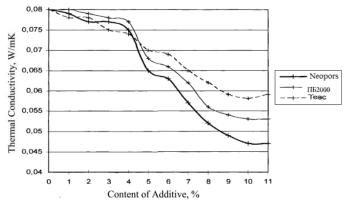
Fig. 4 shows a material thermal conductivity on the amount of the additive quantity.
