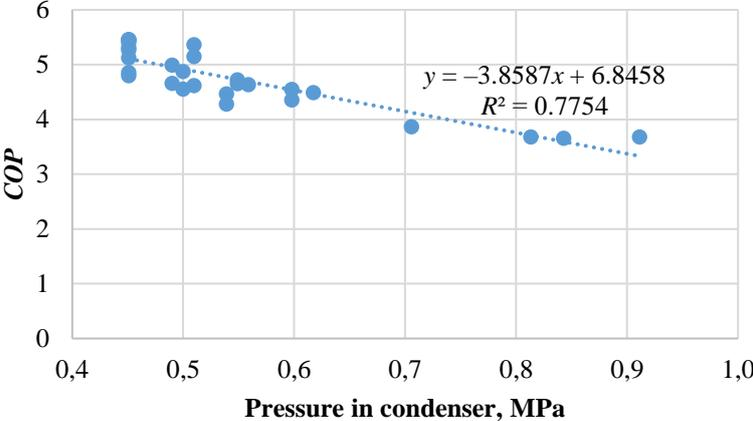
Fig. 2.24. Single-stage compressor *COP* depending on condenser pressure.
