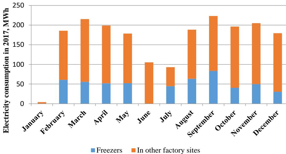
Fig. 2.15. Electricity consumption in fish canning factory.
