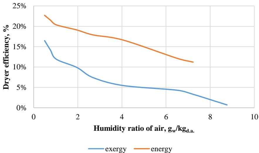
Fig. 2.12. Dryer efficiency versus humidity ratio of drying air.
