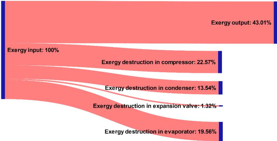
Fig. 2.32. Exergy destruction in two-stage compressor refrigeration system.
