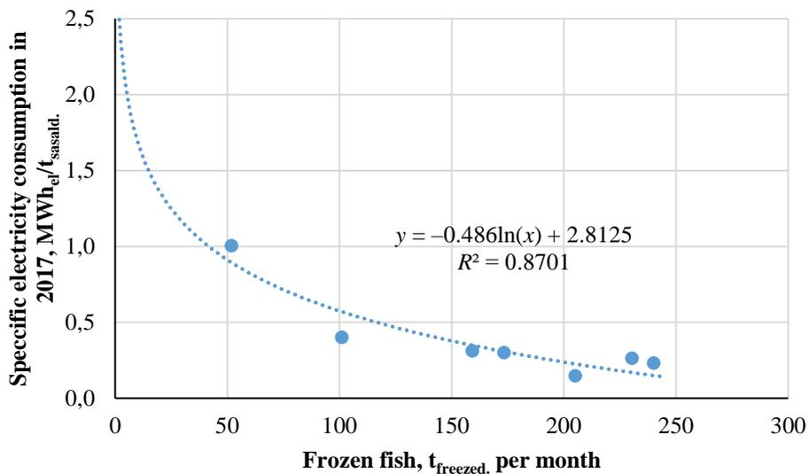
Fig. 2.16. Specific electricity consumption for fish refrigeration.
