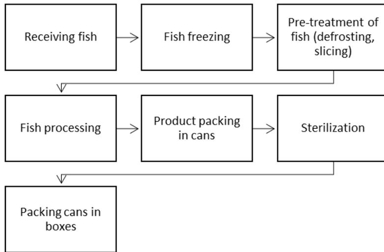
Fig. 2.13. Basic production scheme of canned fish.
