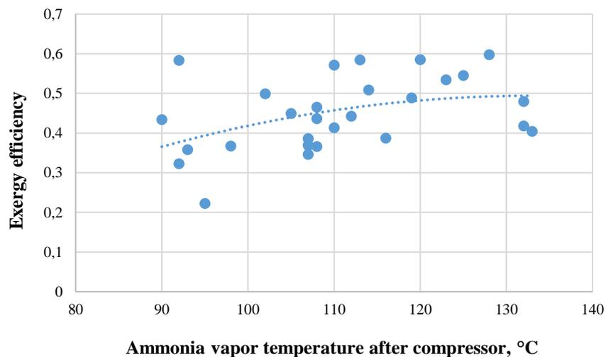
Fig. 2.27. Exergy efficiency of a single-stage compressor refrigeration system depending on ammonia vapor temperature after compressor.
