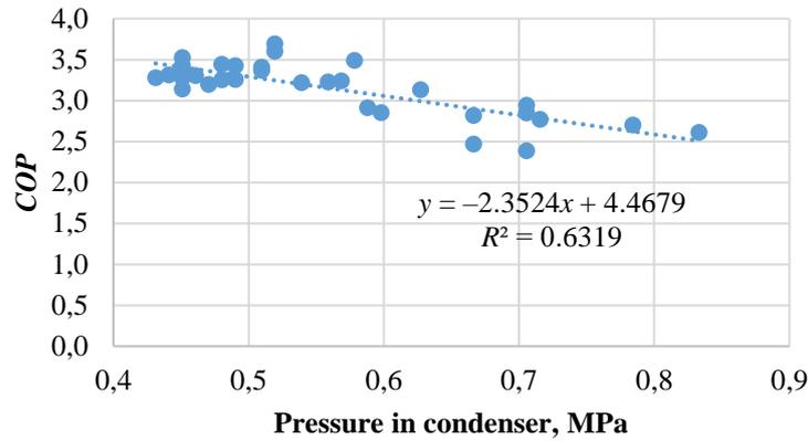
Fig. 2.22. Two-stage compressor *COP* depending on condenser pressure.
