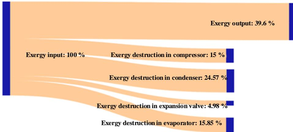
Fig. 2.29. Exergy destruction in single-stage compressor refrigeration system.
