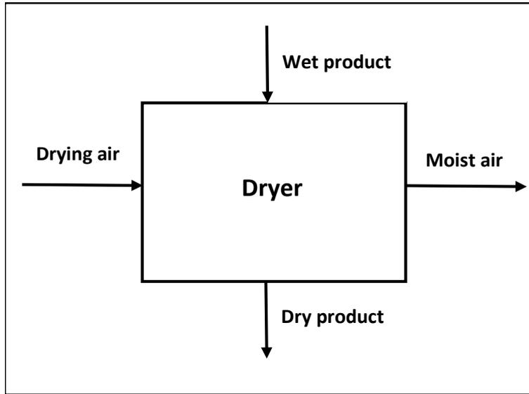
Fig. 2.10. Drying process with input and output terms.
