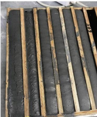
Fig.2 a) Sample lanes in molds, dimensions 30x30x450 mm
