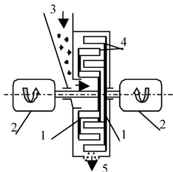
b) Schematic representation of the disintegrator equipment: [2] 1 – rotors; 2 – electric drives; 3 – material supply; 4 – grinding elements; 5 – output
