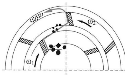
c) Principal scheme of process of raw material milling (longitudinal section) [2], where  $\omega_1$ ,  $\omega_2$  – radial velocity of disintegrator wheels.
