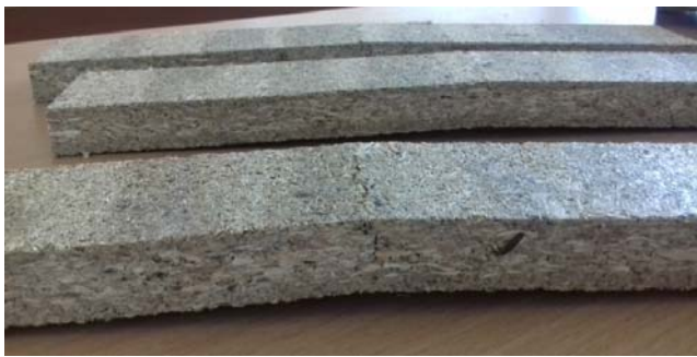
Figure 3 Bending strength test: particle board of wood with hemp chaff fracture
