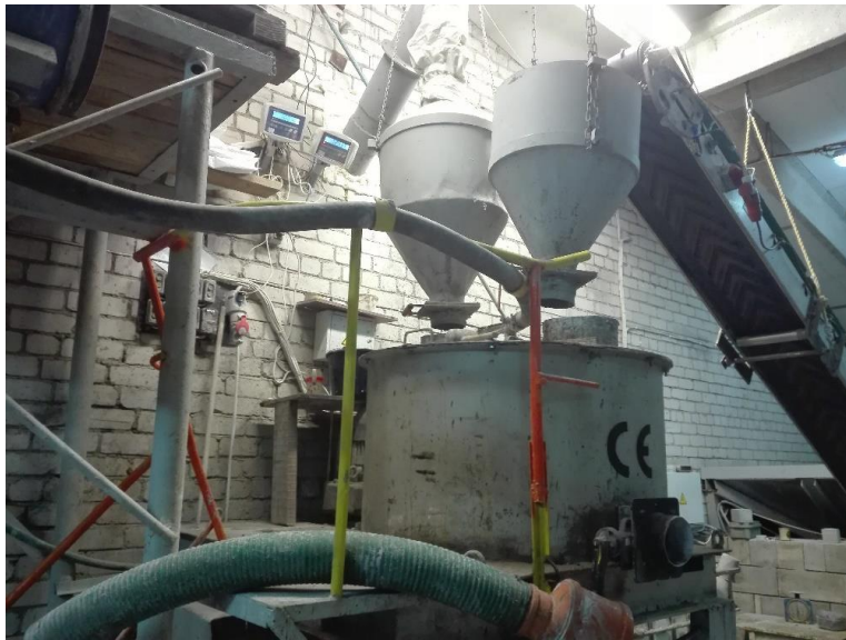
Fig. 1. Turbulence mixer with cavitation effect in the foam concrete plant (intensive mixing technology).
