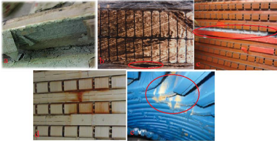
Fig. 2.1. Common generator stator defects [13], [15].
