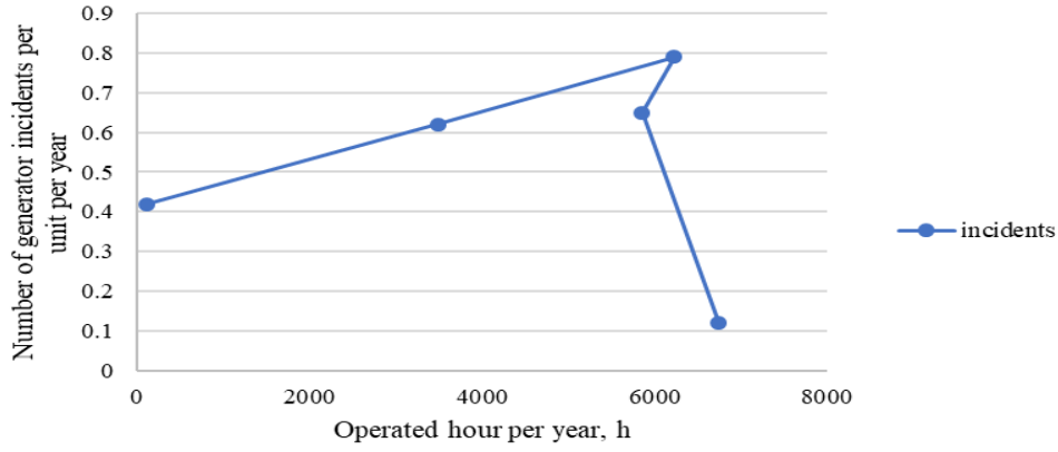
Fig. 3.1. Number of generator system incidents per year per unit relation to operating hours per year.
