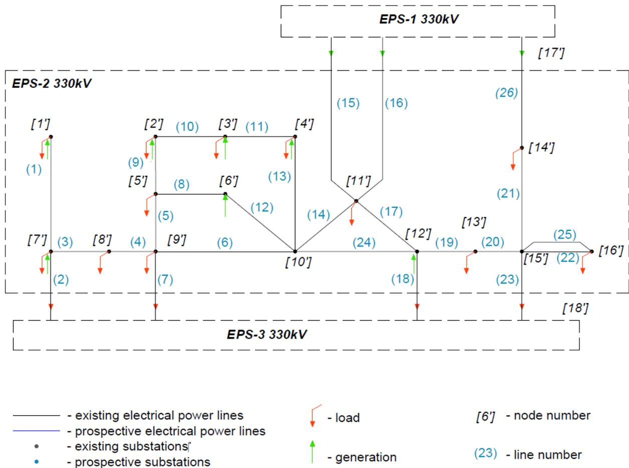
Fig. 3.2. The studied EPS 330 kV model (for Scenario 1).
