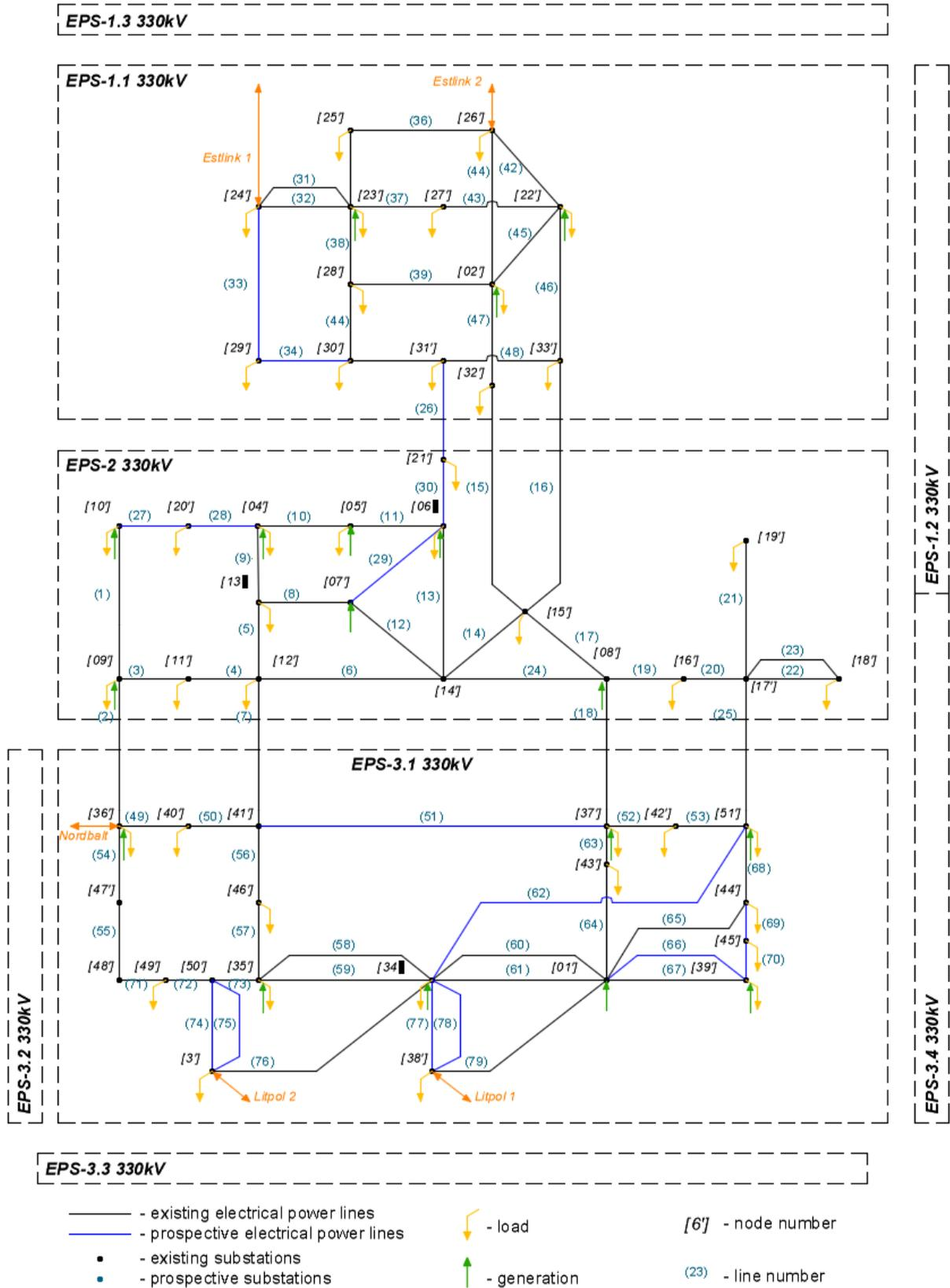
Fig. 3.8. The studied EPS 330 kV model for Scenario 5.
