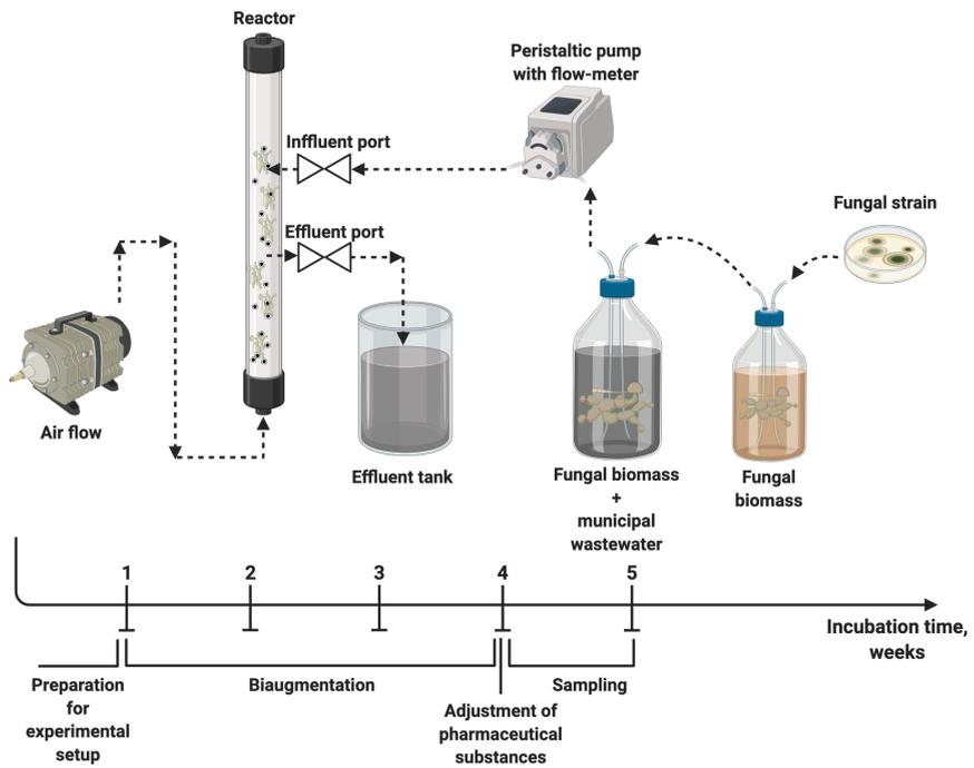
**Figure 1.** A conceptual scheme of a fungal fluidized bed pelleted bioreactor and experimental setup (created with BioRender.com).
