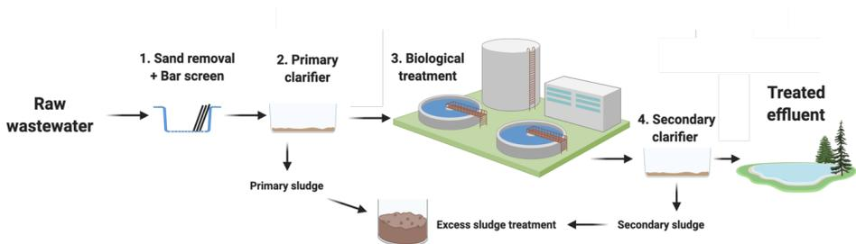
**Figure 2.** Conceptual scheme of a conventional wastewater treatment plant with biological treatment (created with BioRender.com).
