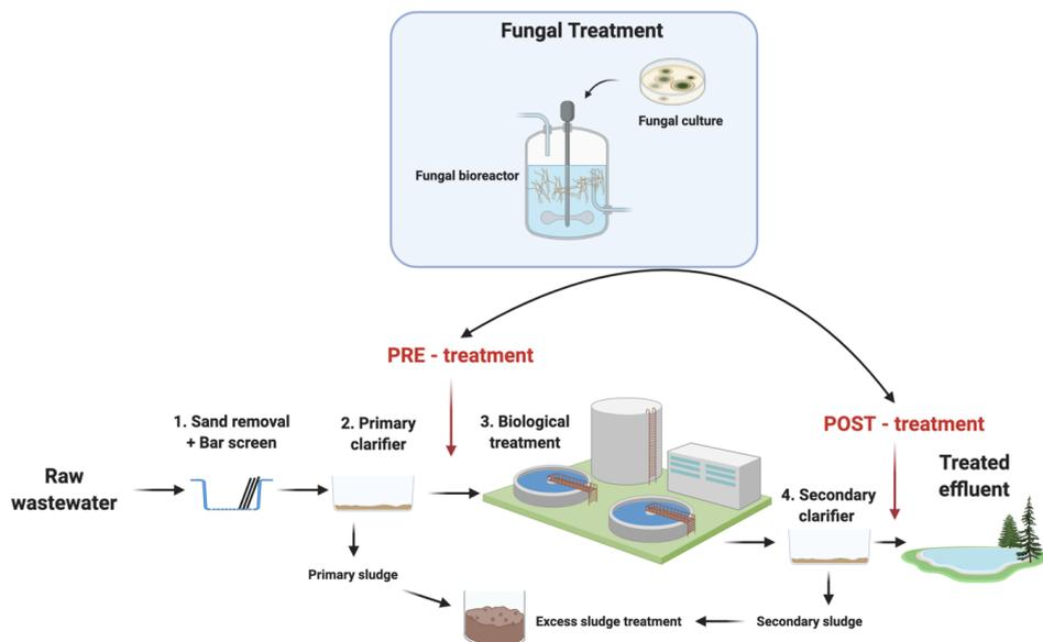
**Figure 7.** Scheme of fungal application in conventional wastewater treatment system (created with BioRender.com)
