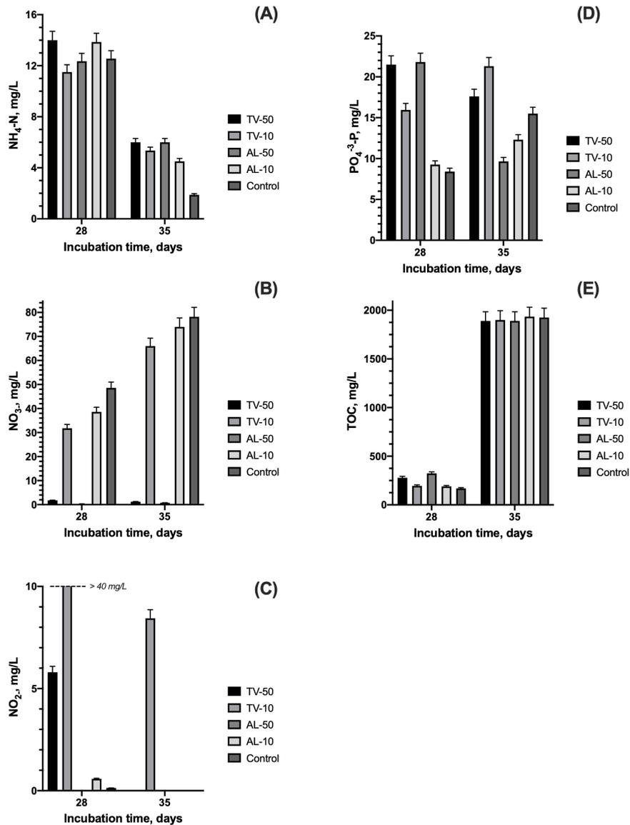
**Figure 6.** The reduction of **(A)** NH<sub>4</sub>-N, **(B)** NO<sub>3</sub>-N, **(C)** NO<sub>2</sub>-N; **(D)** PO<sub>4</sub><sup>-3</sup>-P; and **(E)** TOC by *T. versicolor* (TV) and *A. luchuensis* (AL) in fluidized bed pelleted bioreactor after addition of pharmaceutical substances and bioaugmentation.
