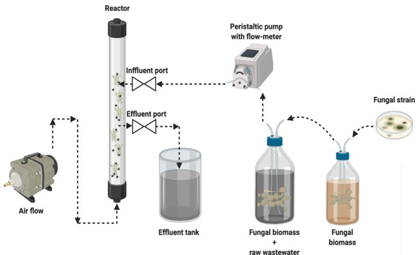
**Figure 10.** A scheme of a fungal fluidized bed pelleted bioreactor (created with BioRender.com)
