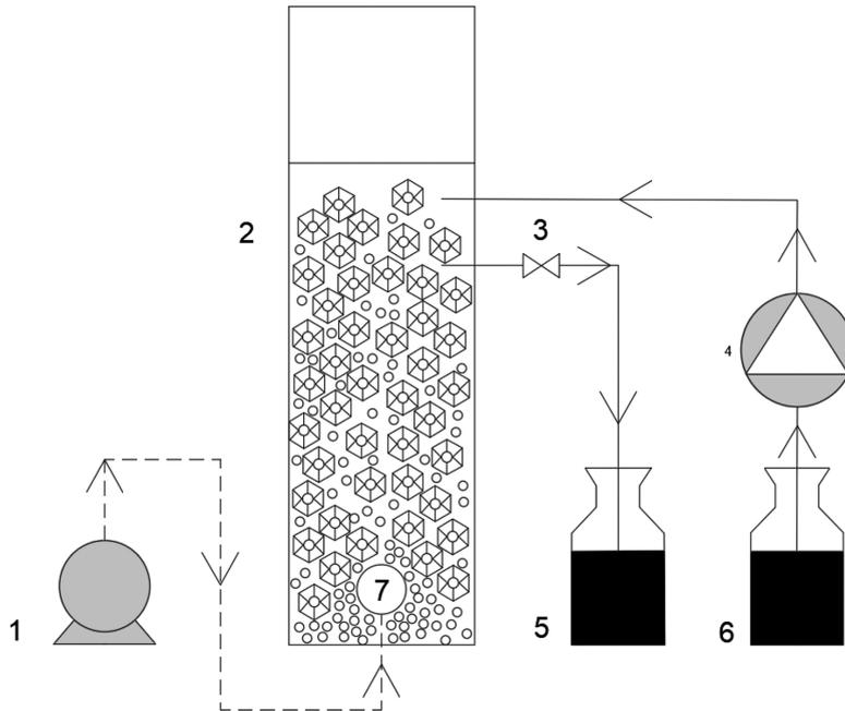
**Fig. 1.** A scheme of a fungal fluidized bed pelleted bioreactor. (1) Air flow; (2) Reactor; (3) Effluent port; (4) Peristaltic pump and flow-meter; (5) Effluent tank; (6) Fungal biomass tank; (7) Reactor with carriers.
