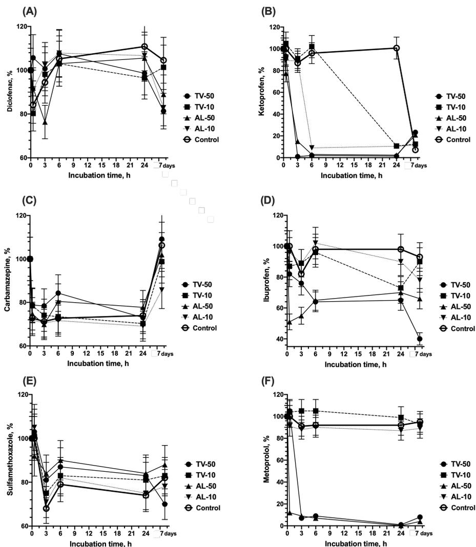
**Figure 5.** The removal efficiency (%) in fluidized bed pelleted bioreactor for incubation time of 7 days of pharmaceutical substances (A) diclofenac, (B) ketoprofen, (C) carbamazepine, (D) ibuprofen, (E) sulfamethoxazole, and (F) metoprolol by *T. versicolor* (TV) and *A. luchuensis* (AL) after 24 h of the final addition of 10 and 50 g wet biomass.
