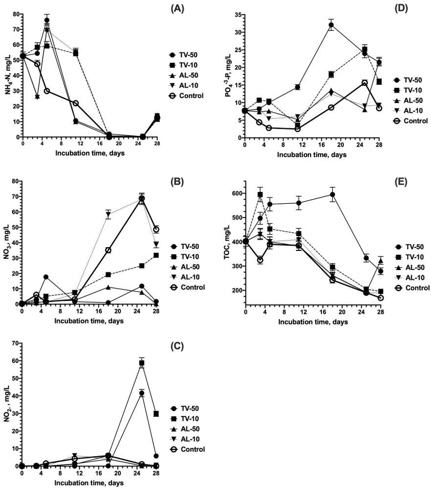
**Figure 2.** The reduction of (A) NH<sub>4</sub>-N, (B) NO<sub>3</sub>-N, (C) NO<sub>2</sub>-N, (D) PO<sub>4</sub><sup>3-</sup>-N, and (E) TOC by *T. versicolor* (TV) and *A. luchuensis* (AL) in fluidized bed pelleted bioreactor.
