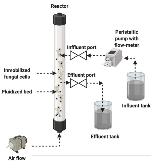
**Figure 6.** The schematic diagram of the fluidized-bed bioreactor system (adapted from Xiao- Ming et al. (2010), (created with BioRender.com))
