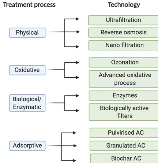
**Figure 3.** Schematic characterization of advanced treatment technologies for wastewater (adapted by the Swedish Environmental Protection Agency (Naturvårdsverket, 2017), (created with BioRender.com))
