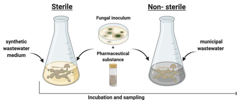
**Figure 8.** Batch experiment with fungi (created with BioRender.com)
