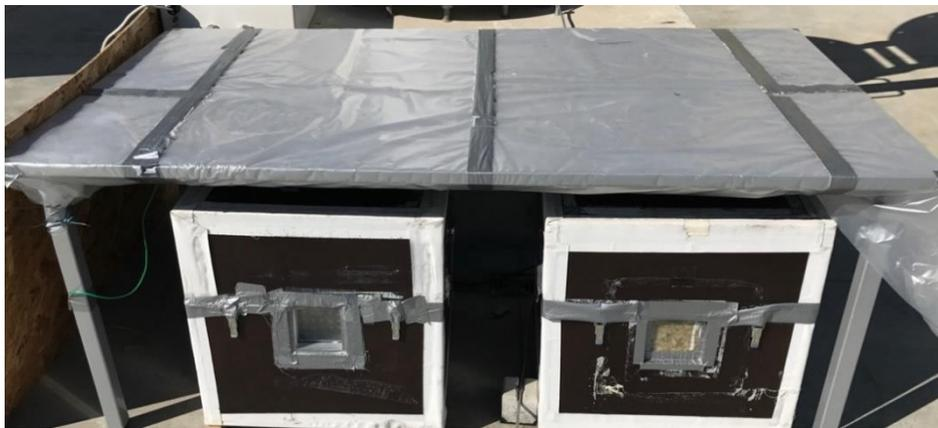
Fig. 1.3. Experimental test box with the facade module (left) and reference box without facade module (right).
