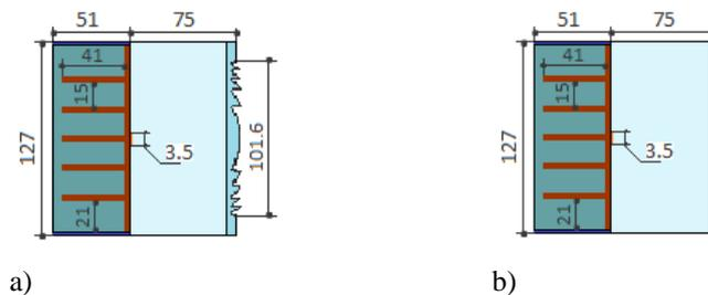
Fig. 1.1. Cross section of the test module with a) Fresnel lens and b) PMMA acrylic glass.
