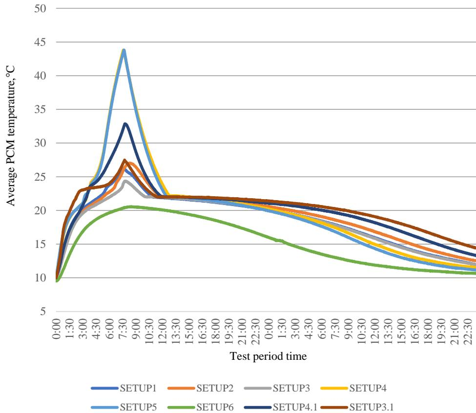
Fig. 2.5. Average PCM temperature in various setups, °C.
