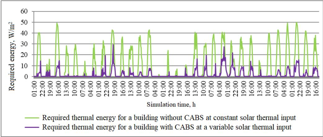
Fig. 2.7. Required energy with and without CABS in July.
