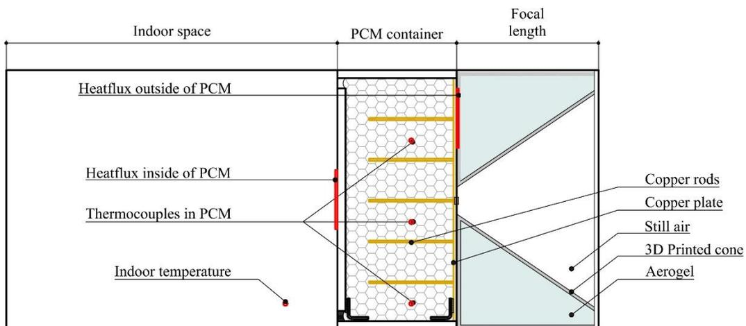
Fig. 1.8. Monitoring equipment scheme.
