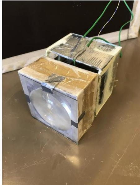
Fig. 1.4. Fresnel lens incorporated in the facade module.
