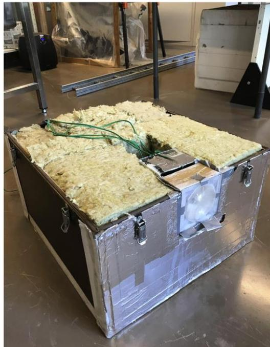
Fig. 1.5. The facade module built in the experimental test box. Total calculated  $U$ -value of the solar facade module is  $0.22 \text{ W}/(\text{m}^2\text{K})$  and of the reference wall  $0.28 \text{ W}/(\text{m}^2\text{K})$ .
