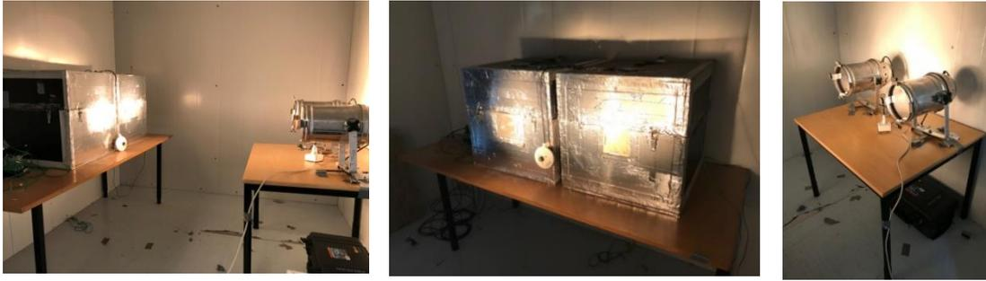
Fig. 1.2. Experimental setup with solar simulator and two test boxes (the reference wall on the right and the wall with test module on the left).
