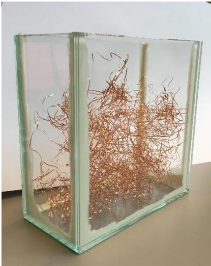
Fig. 1.6. PCM container with fine copper wires as a heat transfer enhancer element.
