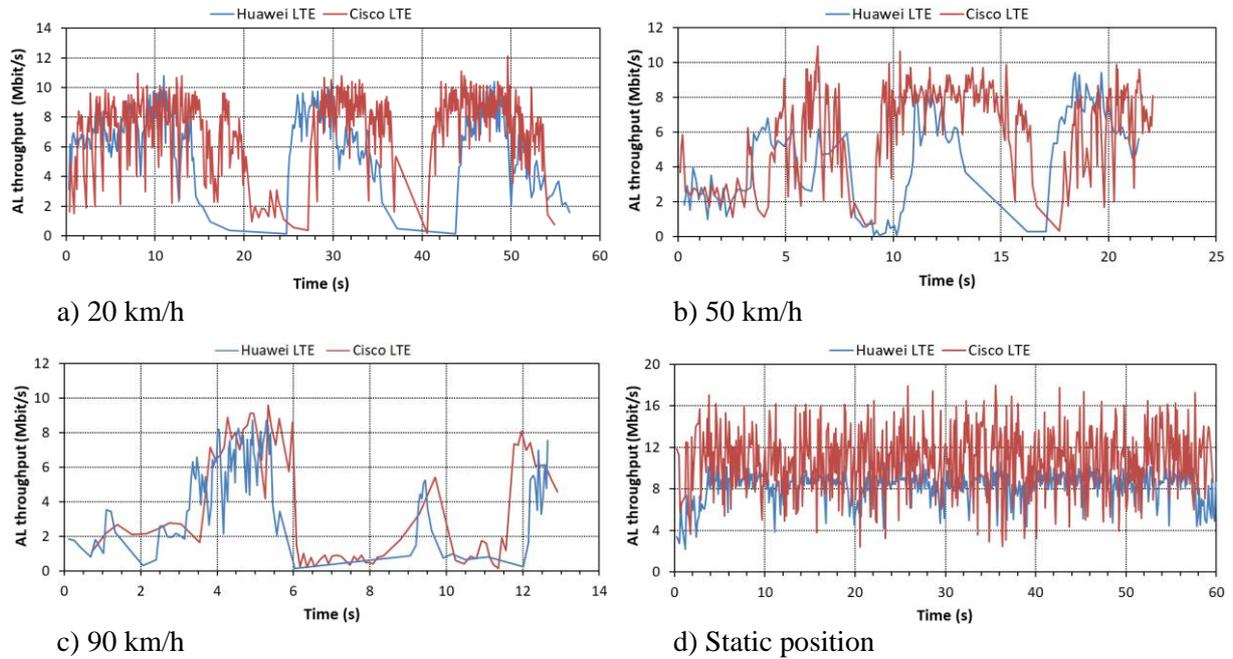
Fig. 4. Comparison of AL throughput using various LTE hardware at various client movement velocities.
