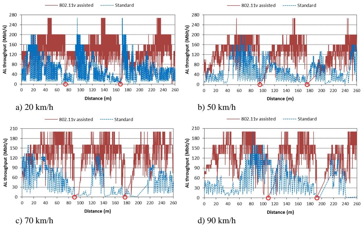
Fig. 14. AL throughput at a velocity of 20 km/h, 50 km/h, 70 km/h, and 90 km/h using 802.11v network assisted and Standard handover methods.
