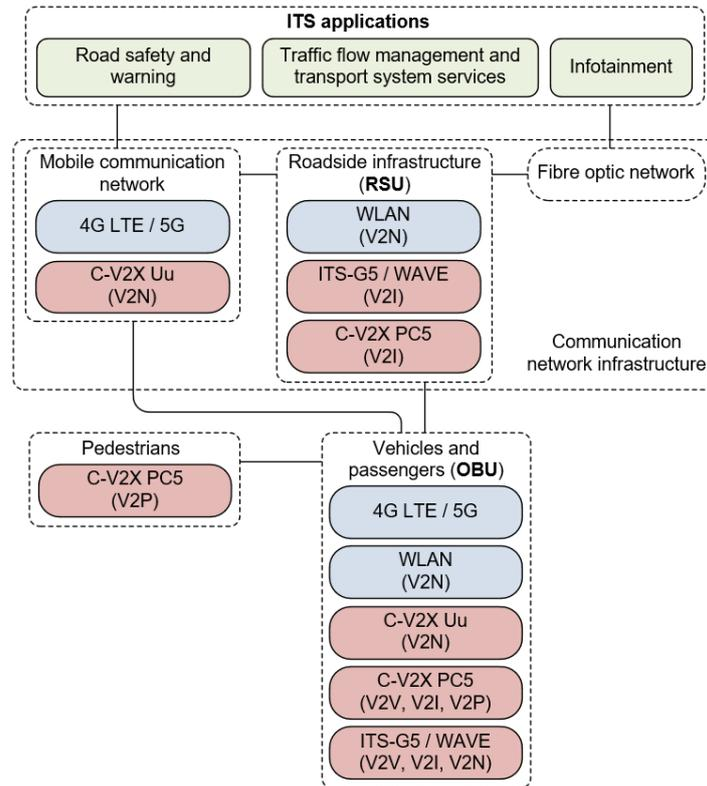
Fig. 2. Combined scheme of ITS communication network technologies.
