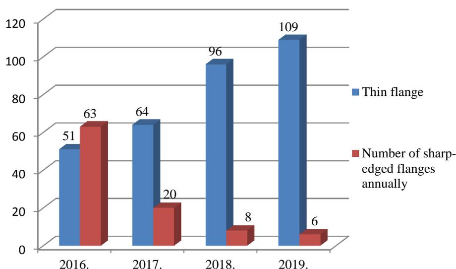
Fig. 4.1. Statistics on sharp-edged and thin flange defects in “Latvijas dzelzceļš” network in 2016–2019.
