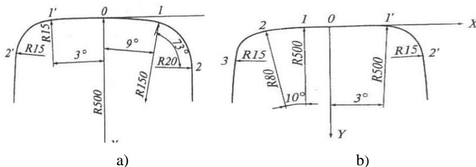
Fig. 4.4. Rail repair profile with vertical wear 1–4 mm and with transmitted tonnage from 150 mil. t. up to 500 mil. t., gross in curves  $R = 800$ – $1000$  m:
