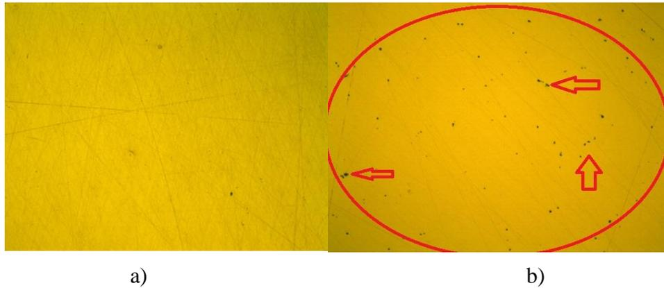
Fig. 3.11. Metal structure of 60 E1 type rail using 50× zoom: a) grinded with a grinding train; b) non-grinded rail.
