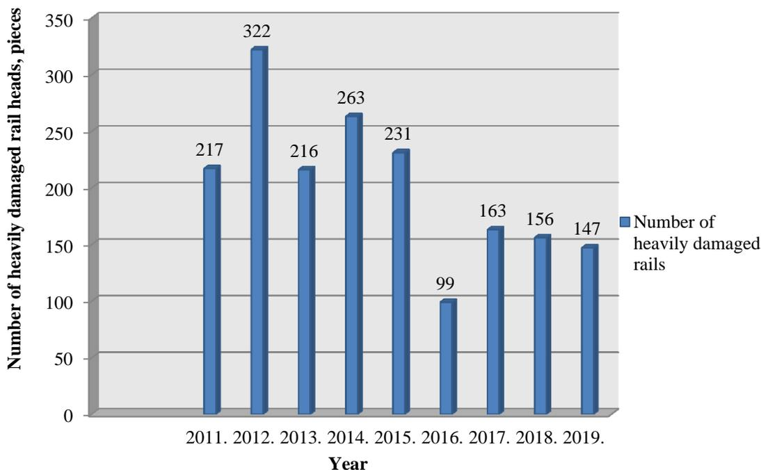
Fig. 2.6. Statistics of heavily damaged rails in “Latvijas dzelzceļš” network from 2011 to 2019.
