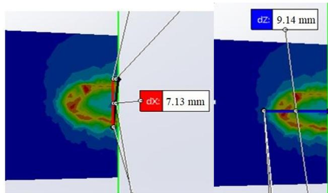
Fig. 5.8. Calculated values of contact area on rail running surface.
