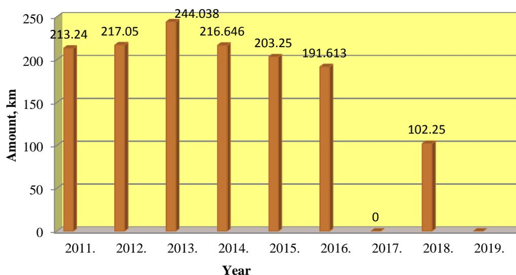
Fig. 2.7. Statistics of quantity (km) of the work of rail grinding train of company “Speno” on Latvian railways in time period 2011–2019.
