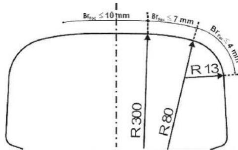
Fig. 4.7. Allowable values of rail 60 E1 type grinding [23].
