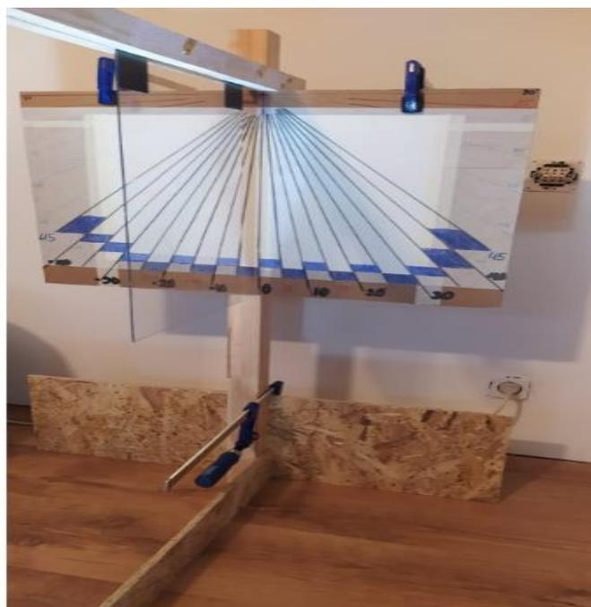
Fig.6.12 Motion of the oscillating pendulum-experimental setup.
