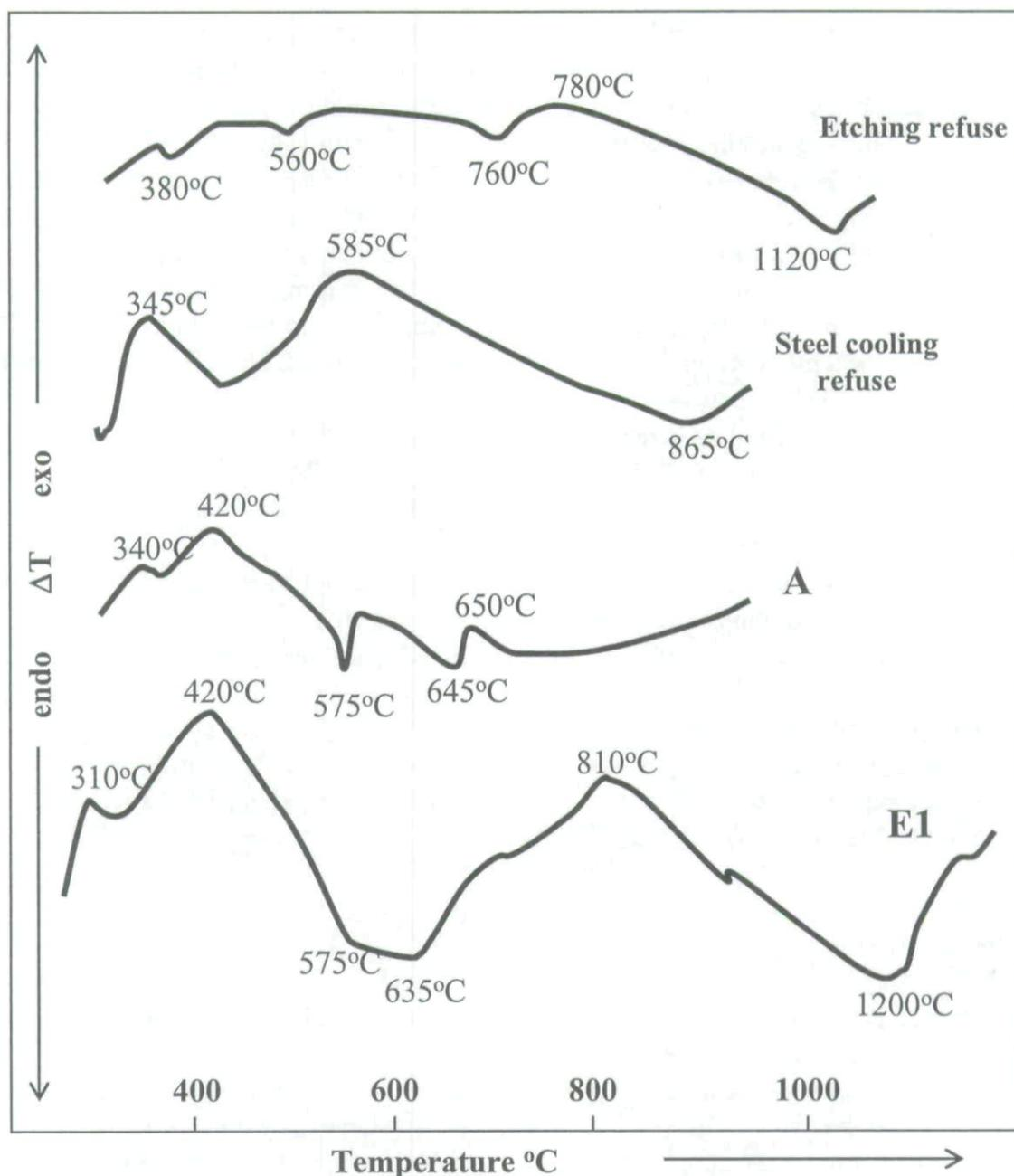
Fig. 1 DTA curves for etching refuse, steel cooling refuse and powder samples of two different compositions studied
