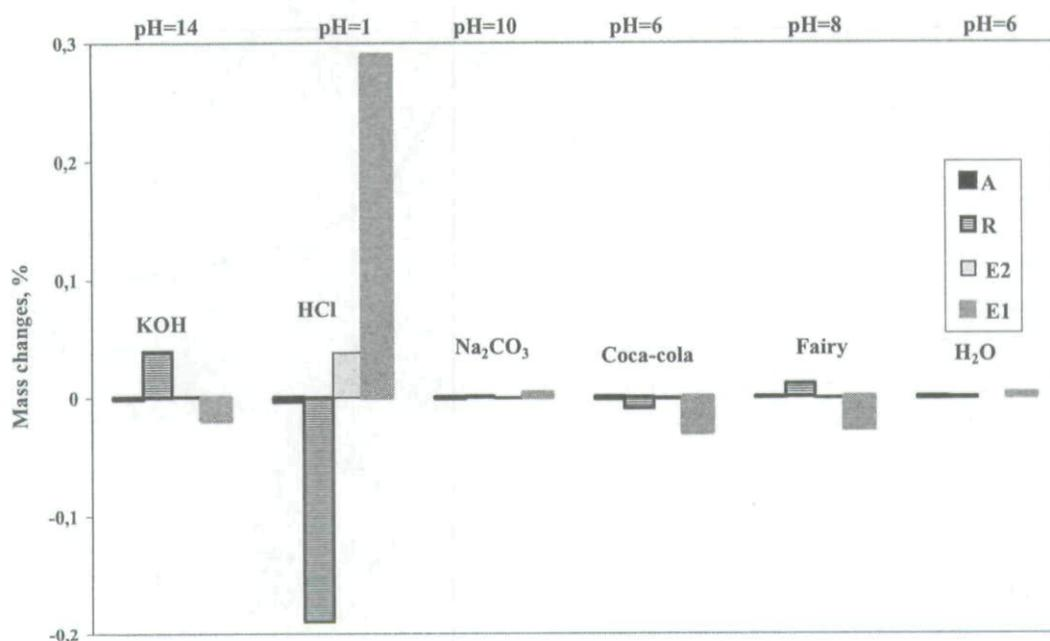
Fig. 3. Mass changes for compositions A, R, E1 and E2 after their treatment in test solutions for 28 days
