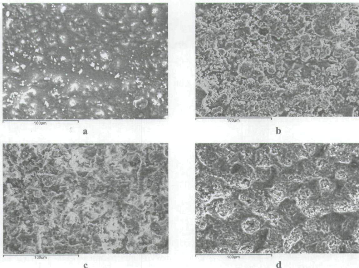
**Fig. 5.** *Microstructure of materials E1 and R, a and c – untreated samples; b and d – after treatment in 3 % HNO<sub>3</sub> test solution*
