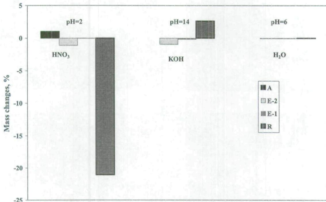
Fig. 4. The mass changes for materials A, R, EI and EII after treatment in the test solutions 3 % HNO<sub>3</sub>, 3 % NaOH and distilled H<sub>2</sub>O
