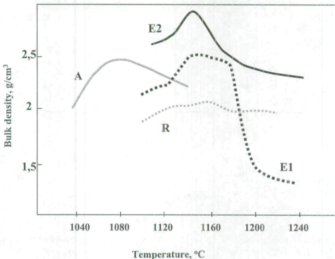
**Fig. 2.** The bulk density of glass-ceramics A, R, E1 and E2 versus sintering temperature
