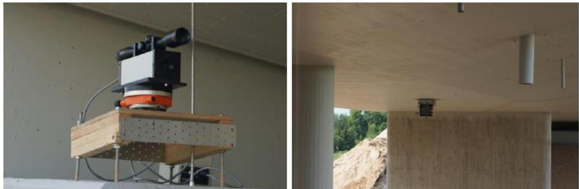
Fig. 1.2. The Noptel PSM-200 displacement sensor is installed on the bridge before performing a dynamic load test.
