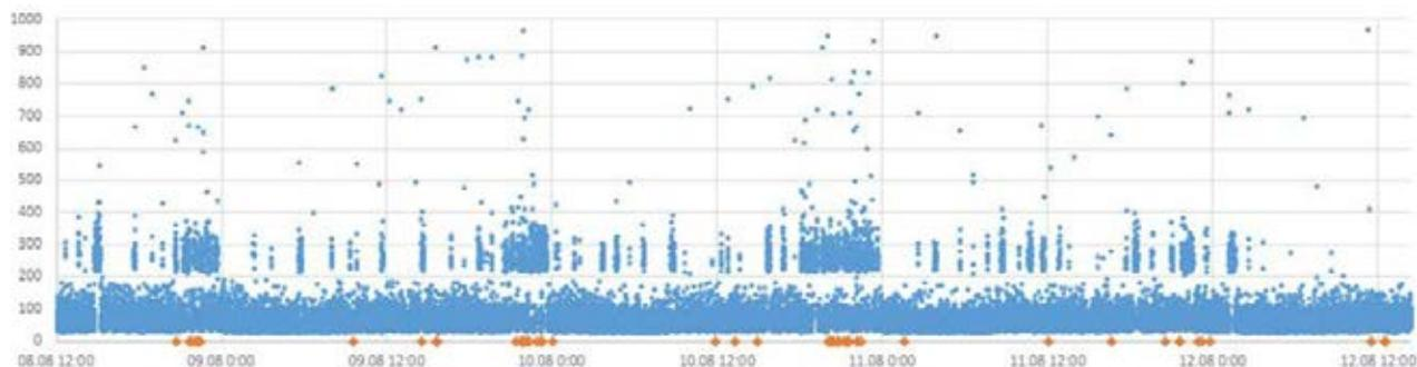
Fig. 2.17 RTT in time of heavily loaded 3G network of the second endpoint (Tele2-LV), ms.
