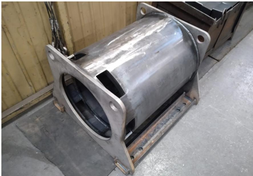
Figure 4-1 – SynRM Housing in Production.
