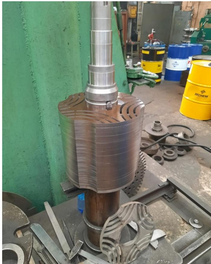
Fig. 4.4. Rotor lamination stack assembly on a shaft.
