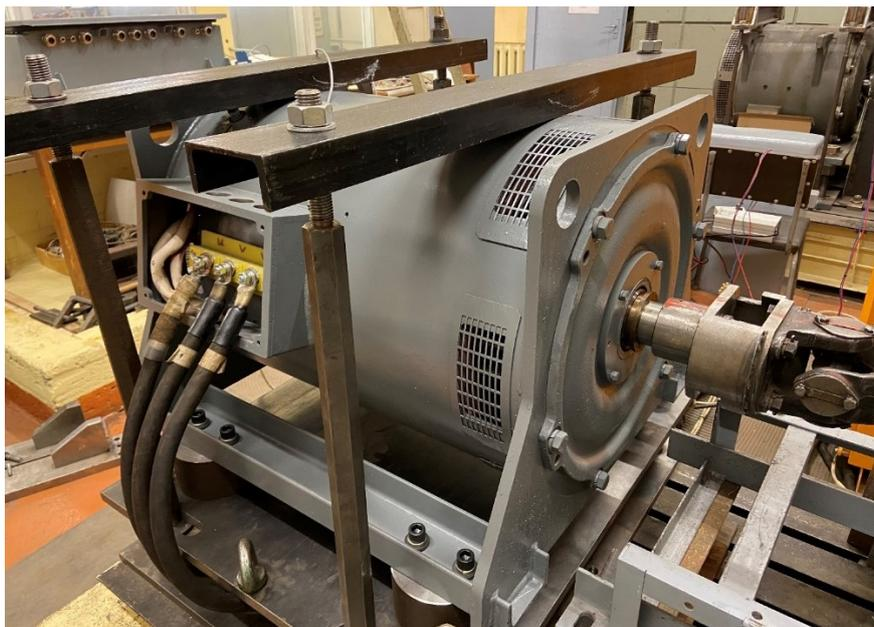
Fig. 4.6. SynRM traction drive on a test-bench.
