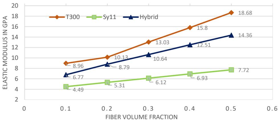
Fig. 3. SolidWorks results of composites: elasticity v/s fiber volume fraction
