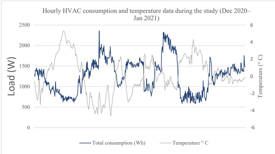
Fig. 4.2. Hourly HVAC consumption and temperature data during the study. Temperature data source [91]
