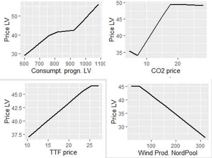
Fig. 3.2. Output of regression analysis using consumption prognosis, CO<sub>2</sub> price, TTF price, and wind production prognosis in Nord Pool as independent variables.
