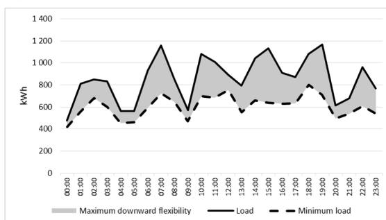
Fig. 4.4. Load profile of the DR resource simulated
