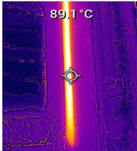
Fig. 5.5. Heating element temperature measurement on Point 7.
