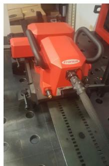
**Fig. 2.2.** Welding tractor
