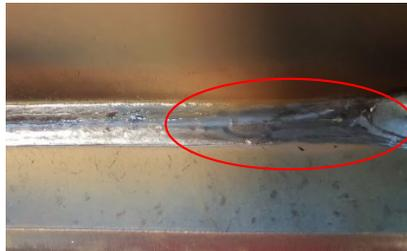
**Fig. 2.6.** Phenomenon of  $\text{SiO}_2$  on the welding seam.
