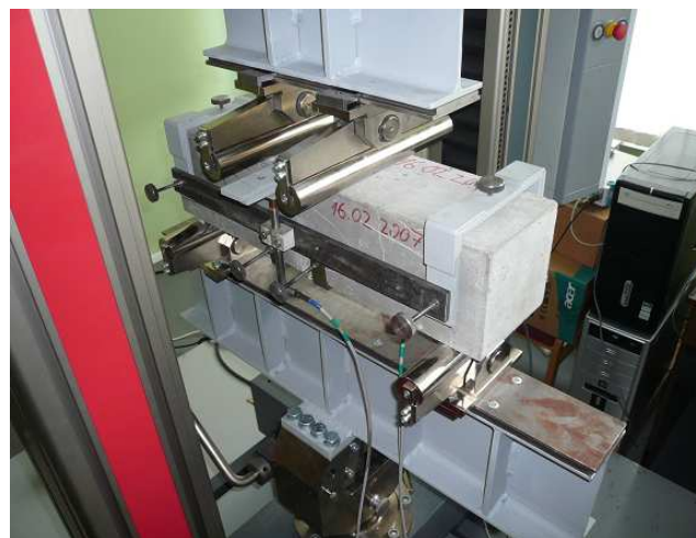
Fig. 6. Fiberconcrete prism under 4-point bending test
