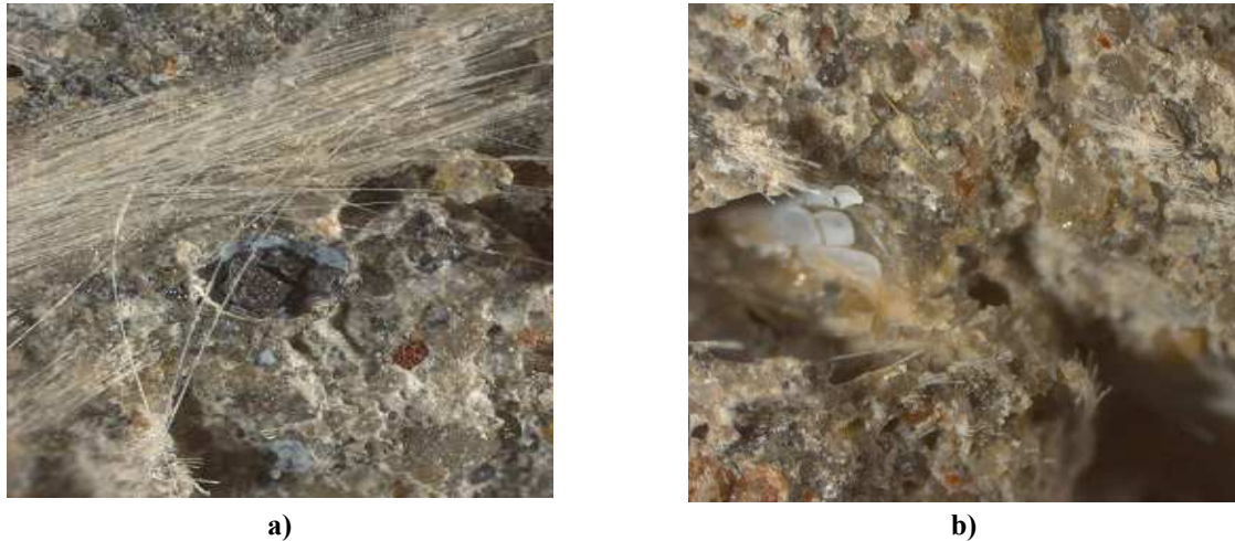
Fig. 5. a) Macro-crack is crossing glass fiber bundle which is laying in crack's plane. Bundle is poorly penetrated by concrete paste (fibers are free of cement paste) and was worked as initial micro-crack in material; b) pulled-out fibers in bundles are crossing crack's plane
