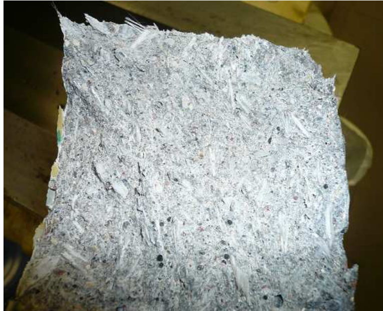
Fig. 8. Crack surface of broken AR-Glass fiber concrete prism
