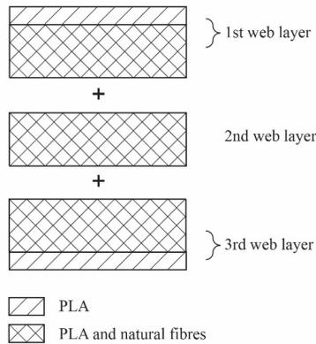
Fig. 2.10. Arranging the fibre layers for the second needle punching.
