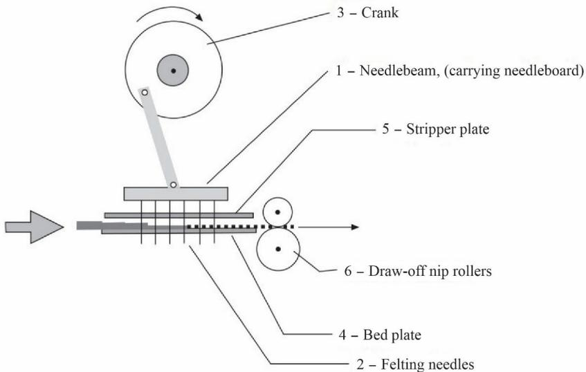
Fig. 2.6. The principle of operation of a simple needle punching machine [34].
