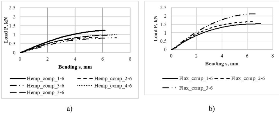
Fig. 3.13. Comparison of load and deflection curves of composite loading tests: a) Hemp\_comp composite samples Hemp\_comp\_1, Hemp\_comp\_2, Hemp\_comp\_3, Hemp\_comp\_4 and Hemp\_comp\_5; b) Flax\_comp composite samples Flax\_comp\_1, Flax\_comp\_2 and Flax\_comp\_3.
