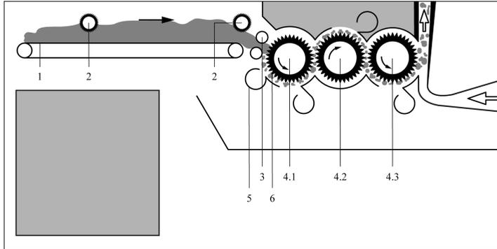
Fig. 2.3. Working principle of the TRÜTZSCHLER CVT3 1200 fibre opening and mixing machine [33].
