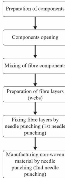
Fig. 2.1. Scheme of nonwoven material production processes.
