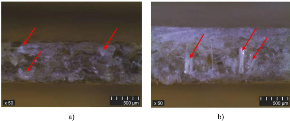
Fig. 3.6. Cross-sections of composite materials: a) Hemp\_comp composite material; b) Flax\_comp composite material.
