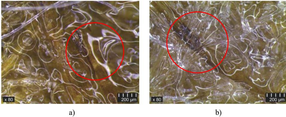
Fig. 3.7. Natural fibres embedded in composite materials: a) hemp fibre in Hemp\_comp composite; b) flax fibre in Flax\_comp composite.
