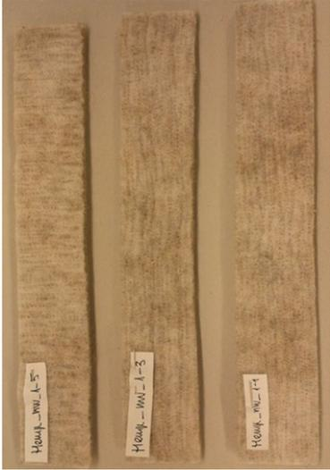
Fig. 3.1. Strips of Hemp\_nw\_1 nonwovens samples.
