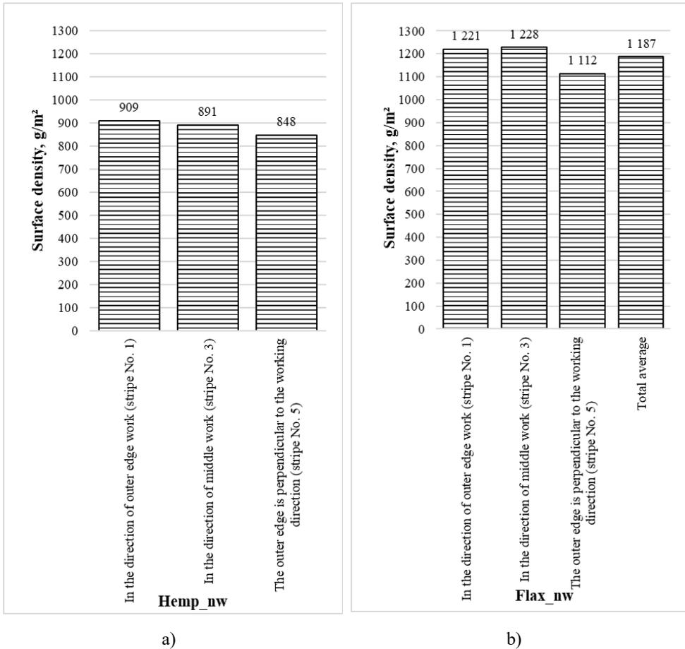
Fig. 3.1. Dependence of nonwovens' surface density on the sample cutting direction:
