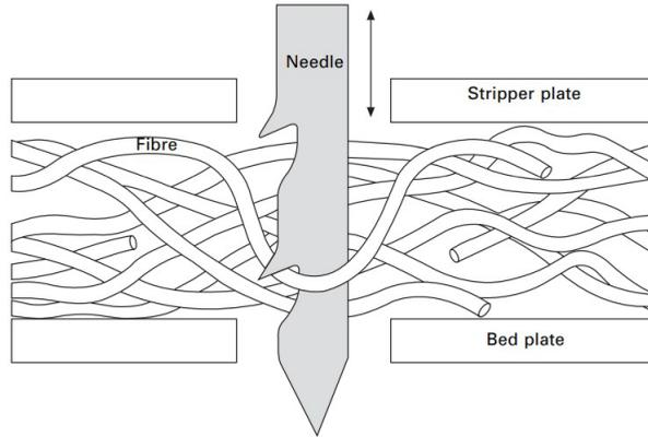
Fig. 2.7. The principle of operation of the needle when punching [34].
