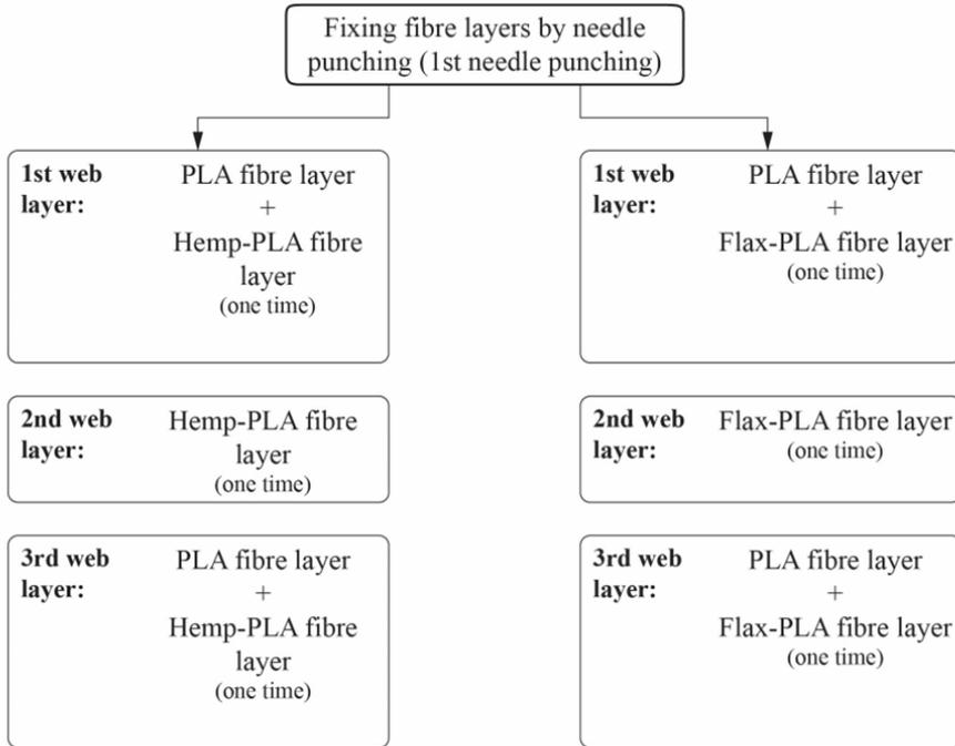
Fig. 2.8. First needle punching of the fibre layers.
