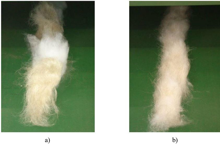
Fig. 2.4. Flax (light brown) and PLA fibres (white) are arranged on the feed belt of the fibre opening and mixing machine.
