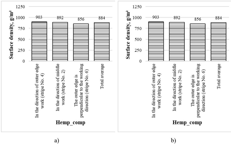
Fig. 3.8. Dependence of the surface density of the composite materials on the cutting direction of the initially made nonwoven material's sample: a) Hemp\_comp; b) Flax\_comp.
