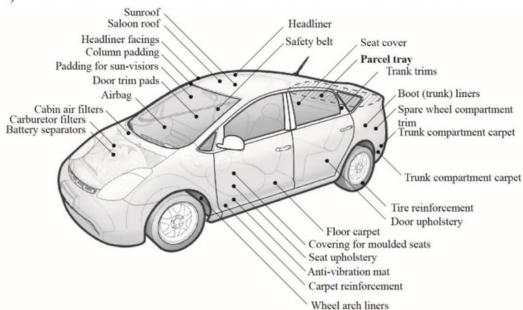
Fig. 1. 1. The structure of the passenger car and its main elements [8].
