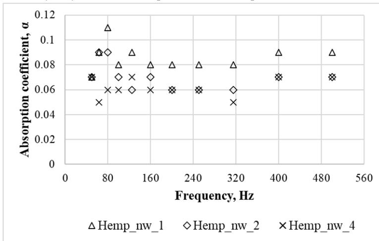
Fig. 3.2. Absorption coefficient values of Hemp\_nw samples in the low frequency radiation range.
