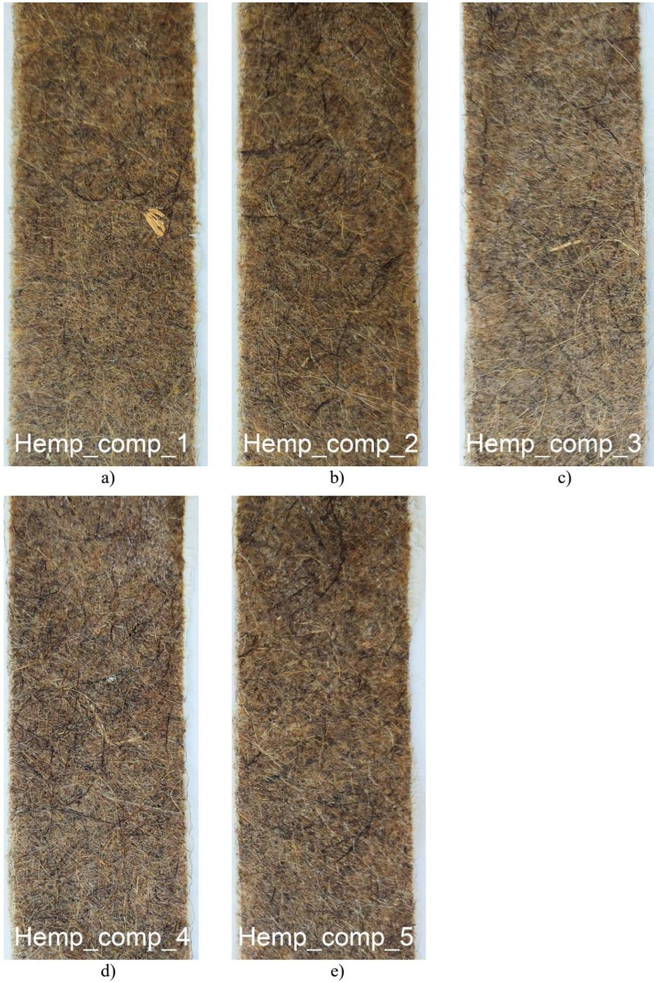
Fig. 3.4. Hemp\_comp composite material sample strips: a) Hemp\_comp\_1; b) Hemp\_comp\_2; c) Hemp\_comp\_3; d) Hemp\_comp\_4; and e) Hemp\_comp\_5.
