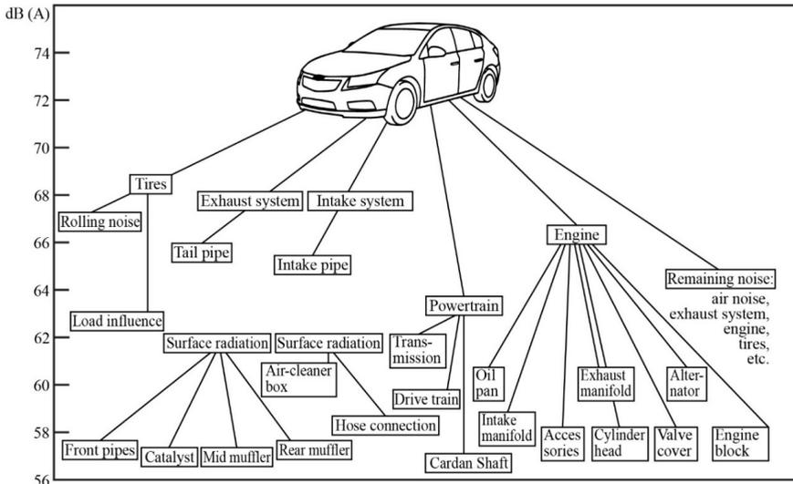
Fig. 1.2. Layout of noise sources according to the noise test of a moving car [13].
