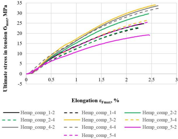
Fig. 3.9. Hemp\_comp composite material in ultimate tensile strength to material collapse for strips Nos. 2 and 4 of samples: Hemp\_comp\_1, Hemp\_comp\_2, Hemp\_comp\_3, Hemp\_comp\_4 and Hemp\_comp\_5.
