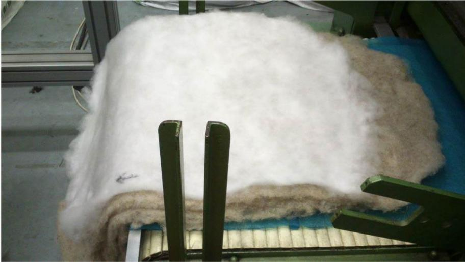
Fig. 2.9. Preparation of all fibre layers for the second needle punching.
