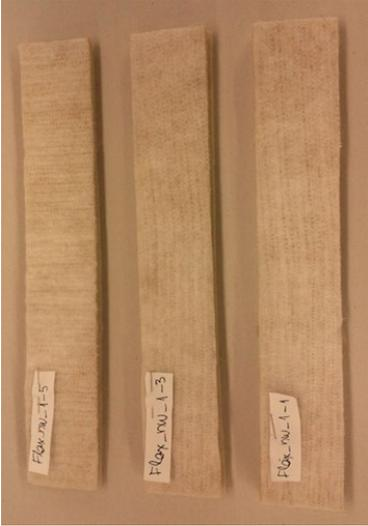
Fig 3.2. Strips of Flax\_nw\_1 nonwovens samples.
