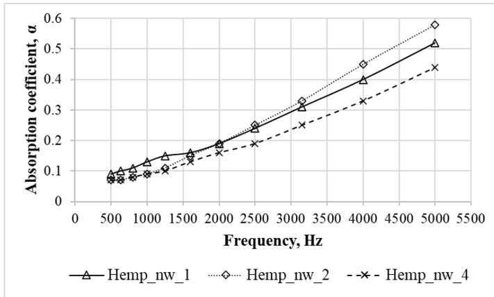
Fig. 3.3. Absorption coefficient values of Hemp\_nw samples in the medium frequency radiation range.
