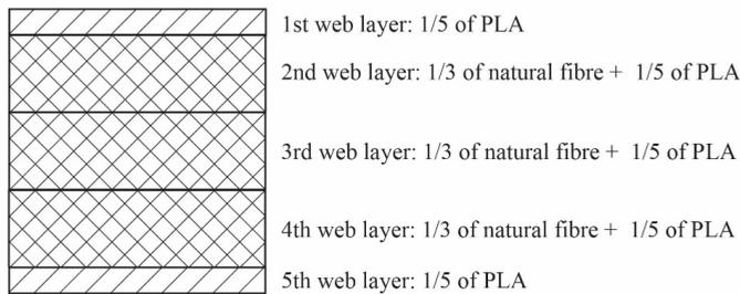
Fig. 2.2. Multilayer structure of nonwoven material.
