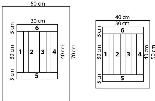
Fig. 2.11. The scheme of cutting out the sample strips: for the Hemp\_nw nonwoven sample (on the left); for the Flax\_nw nonwoven sample (on the right).
