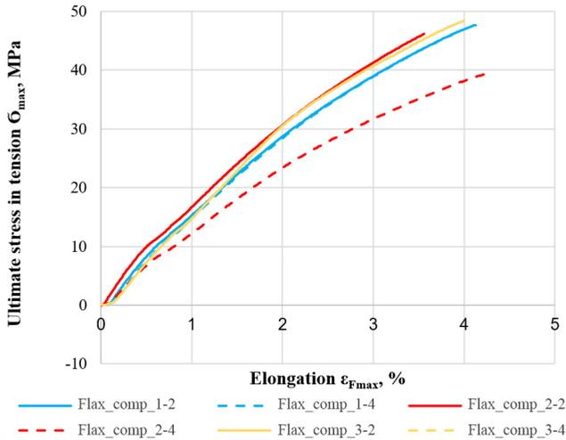
Fig. 3.10. Flax\_comp composite material in ultimate tensile strength to material failure for strips Nos. 2 and 4 of samples: Flax\_comp\_1, Flax\_comp\_2 and Flax\_comp\_3.
