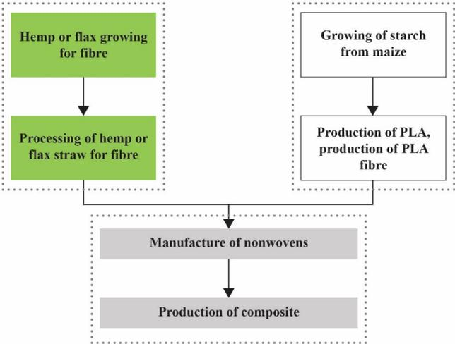
Fig. 2.12. The main stages of composite material production – from the extraction of the fibres forming it to the finished product.
