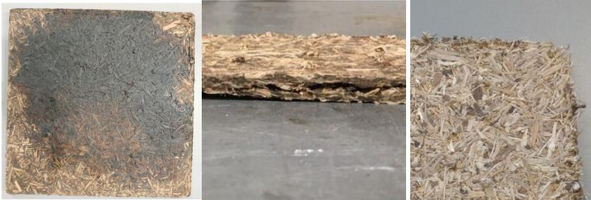
Fig. 2.2. The boards produced under extreme independent variable values.
