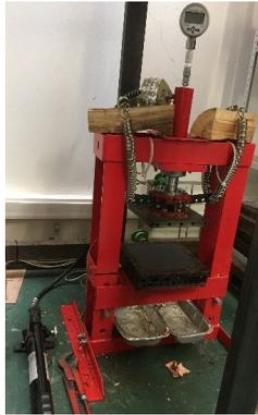
Fig. 1.1. Hydraulic hot press.
