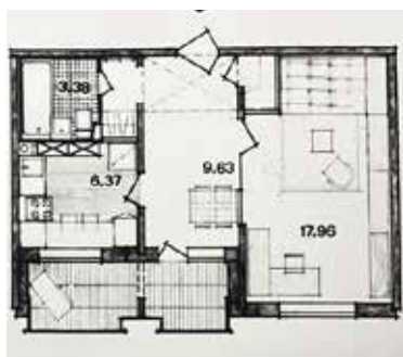
Figure 103. The layout of a one-room apartment in a nine-storey residential building of the 119 series standard project (39.50 m 2 ; 1970s).
