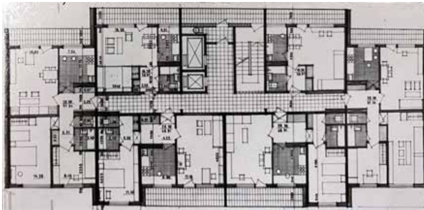
Figure 82. Typical floor plan of sections 1-1-2-2-3-3 of a twelve-storey residential building of the 104 series standard project (1970s).
