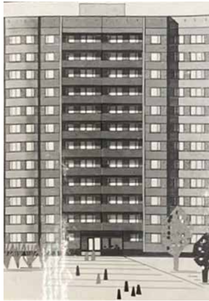
Figure 81. Sketch of a twelve-storey residential building of the 104 series standard project (1970s).
