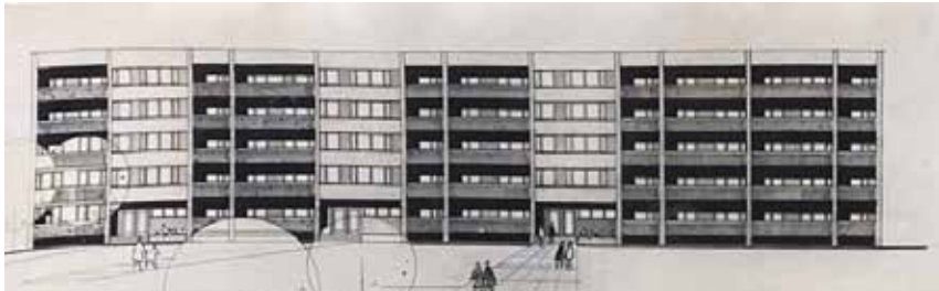
Figure 76. Sketch of a five-storey residential building of the 103 series standard project (1970s).
