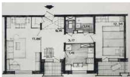
Figure 104. The layout of a two-room apartment in a nine-storey residential building of the 119 series standard project (55.06 m 2 ; 1970s).
