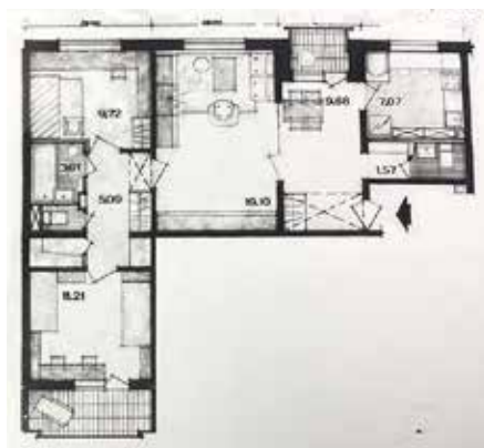
Figure 105. The layout of a three-room apartment in a nine-storey residential building of the 119 series standard project (71.57 m 2 ; 1970s).
