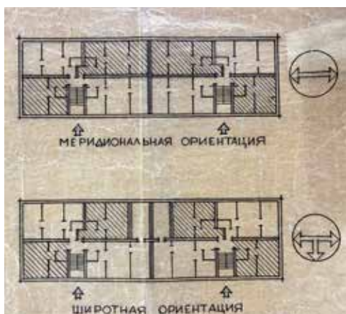
Figure 42. Layout of apartments in a residential building of the 1-316-1 series standard design (1958).
