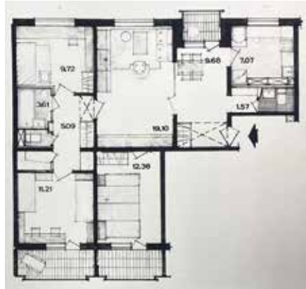
Figure 106. The layout of a four-room apartment in a nine-storey residential building of the 119 series standard project (84.01 m 2 ; 1970s).
