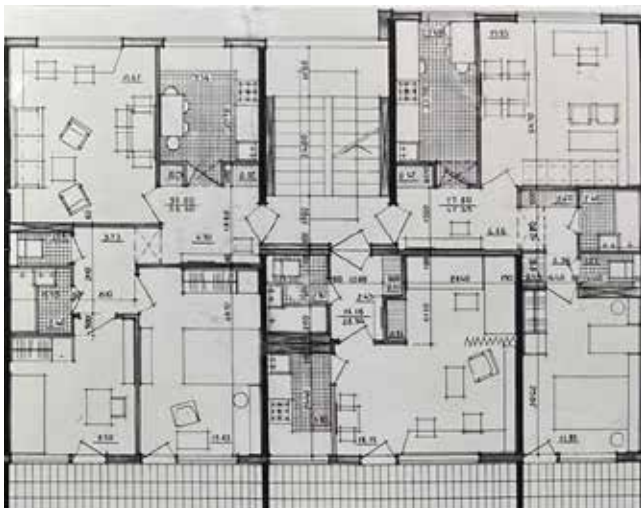
Figure 79. Sketch of a five-storey residential building of the 104 series standard project (1970s).
