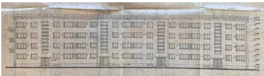
Figure 67. Facade of a residential building (without balconies) of the 1-318A-33/4 series standard project (1964).
