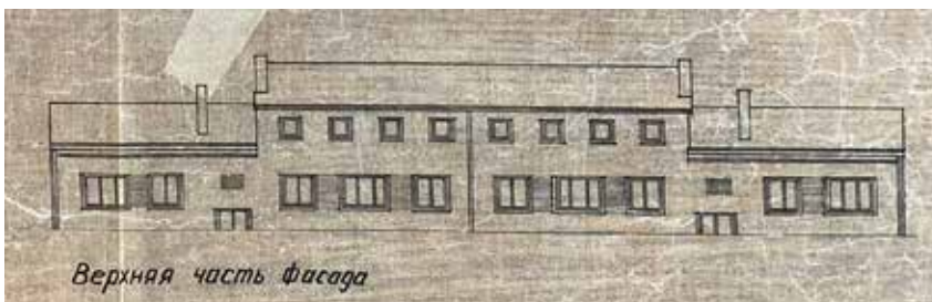
Figure 55. Artists' studio in the central part of the top floor of a residential building of the 1-316 series standard project (1958).
