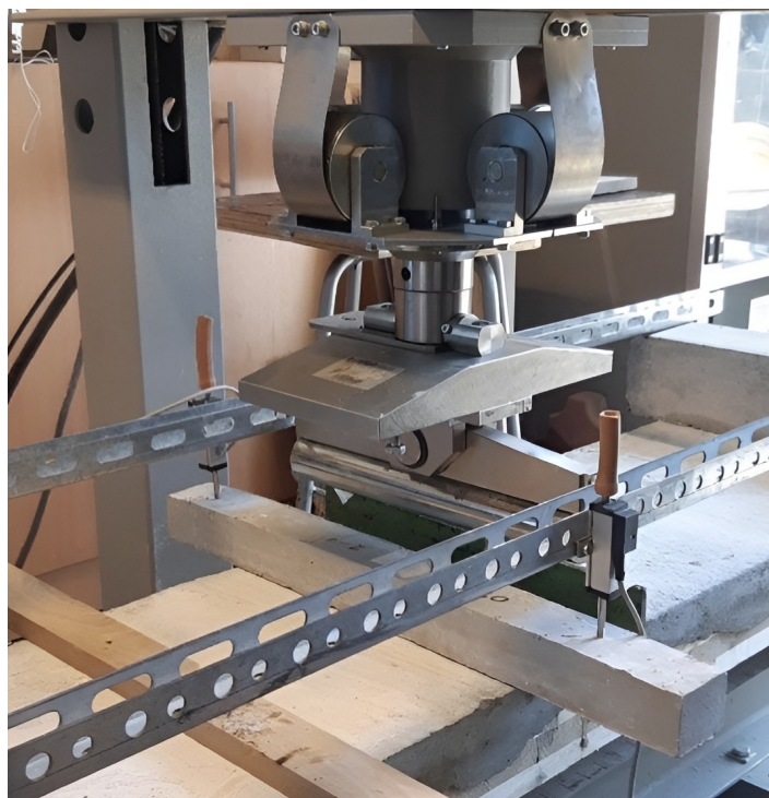
Figure 8. Testing setup with sensors placed 4 cm away from the centre of gravity of the element.
