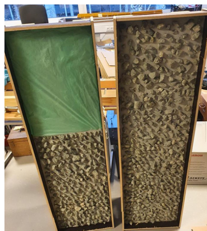
Figure 1. The adhesive granite chips method prepares timber members for connection with the concrete layer.
