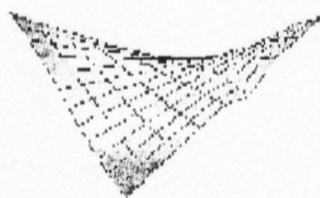
Fig. 6. Experimental mode shape (1, 1) for the first frequency of plate ud1
