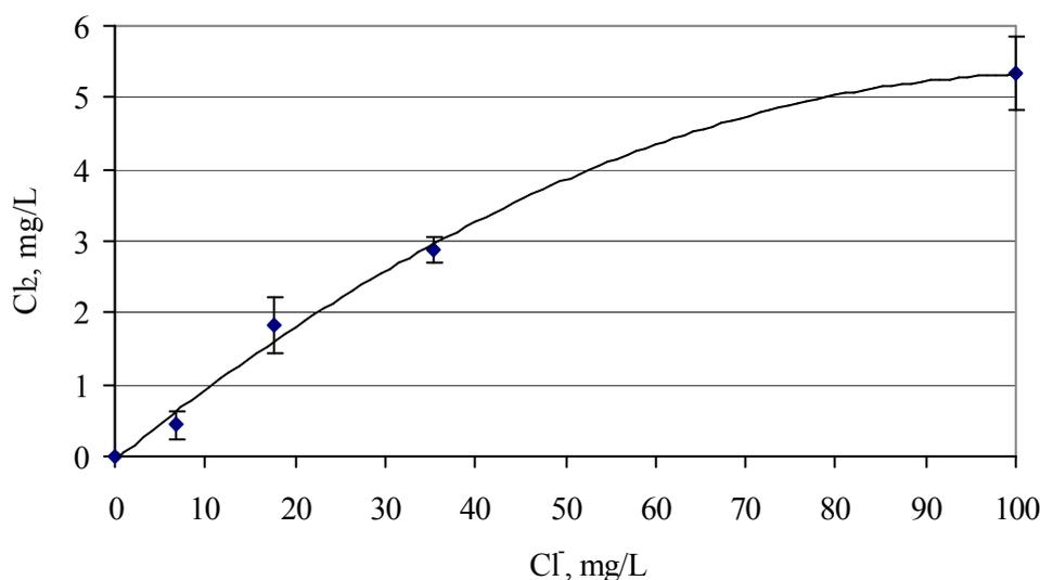
**Figure 2.** Amount of chlorine formed in samples with different initial concentrations of chlorine ions. Electrolysis was carried out in 0.5 L of solution ( $I = 0.1$  A,  $pH 7 \pm 0.2$ ,  $t^{\circ} = 23 \pm 2^{\circ}C$ ,  $t = 15$  min). The results also confirmed that disinfection effect is a result of generation of oxidant species from chlorine rather than effect of electricity *per se*, formation of radicals in water.
