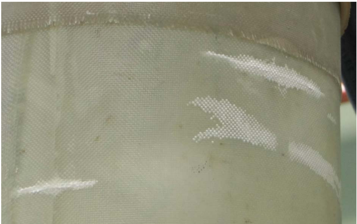
Figure 2.1. The damage of the Type 0 specimen
