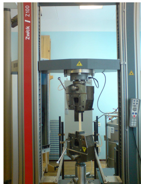
Fig. 4. Specimen tension test on ZWICK Z100
