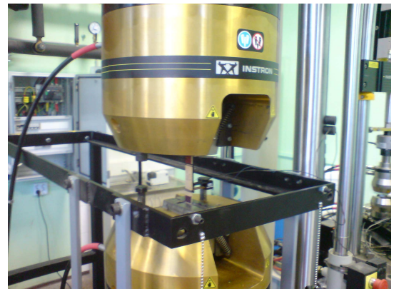
Fig.3. Specimen tension test on INSTRON 8802
